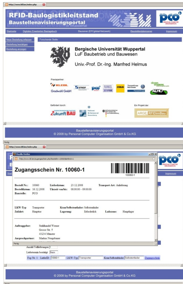
Figure 8: Construction Site (notification) portal for online shipment registration with delivery ID generation (left: Screenshot "Home" and the right screenshot "access permit")
