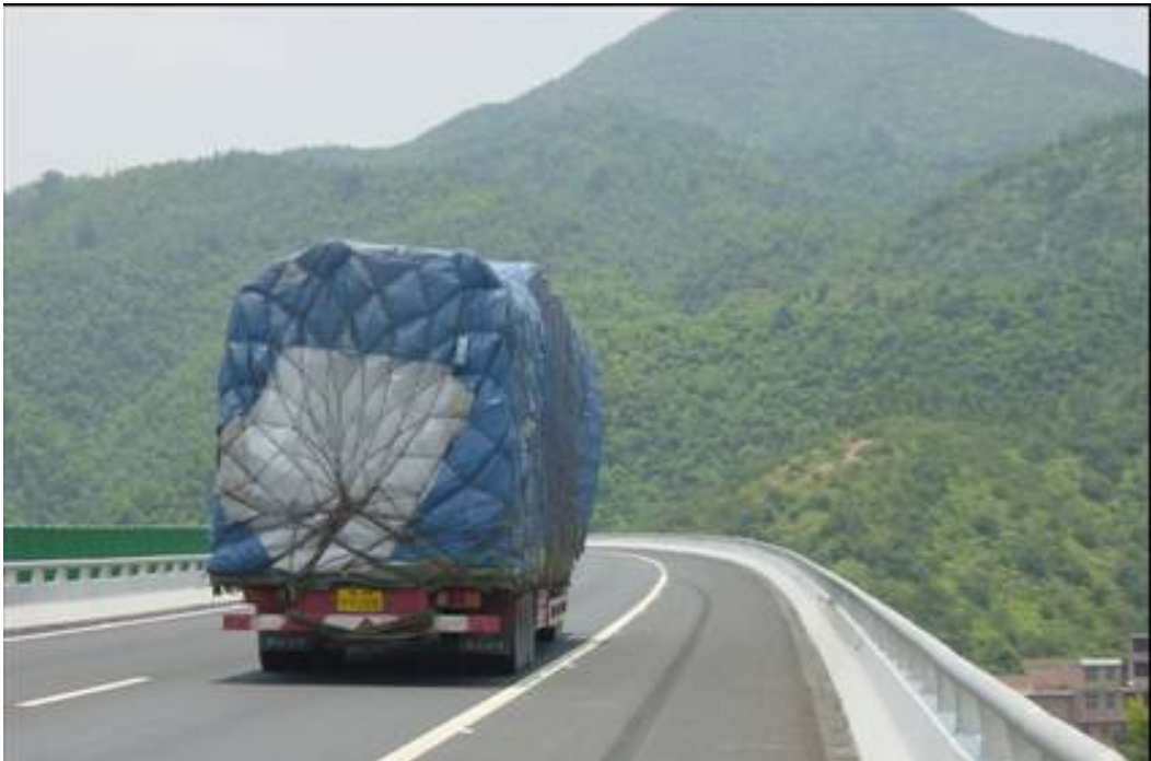
Figure 3. Overloaded Truck on Bridge
