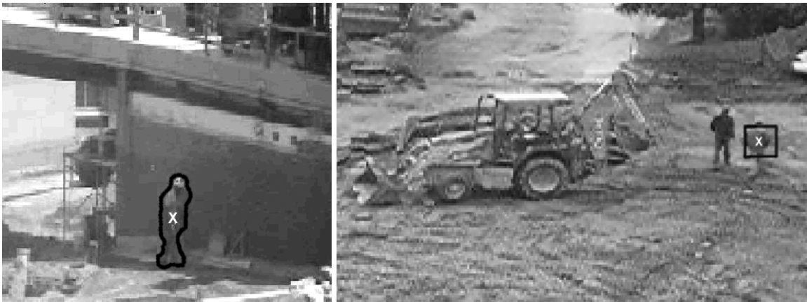
Figure 2. Dynamic Video Camera Tracking of Workers' Shape and Centroid using Feature Detection Algorithm (Teizer and Vela 2008a)
