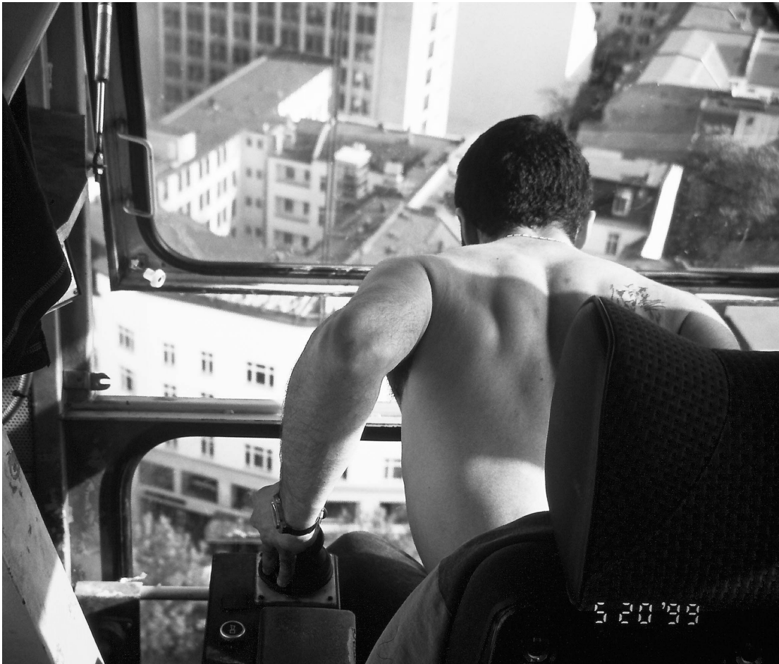
Figure 3. Operator Leaning out of the Window for Better View
