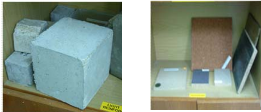
Fig. 5: Wood cement block and particle board made from C & D waste.
