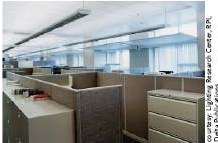
Figure 6, Daylight Harvesting by Using Exterior and Interior Daylight Shelves
