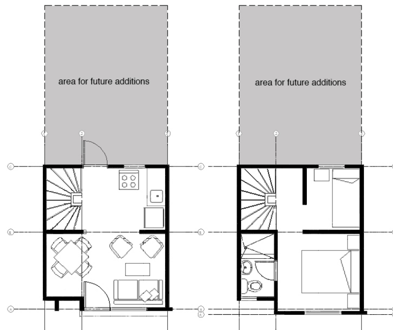
Fig. 4. Plans of first level (left) and second level (right) of the 37 m2 basic unit.
