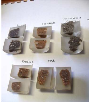
Figure 12. Samples cut and polished (left) and their observation with a binocular amplifying glass (left)
