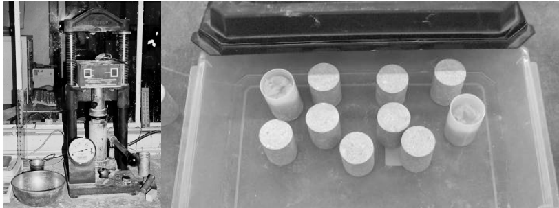
Figures 1 and 2 – Hydraulic press and packing of specimens for tests
