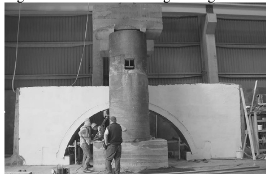
Figure 8: Test set-up for mid-span loading
