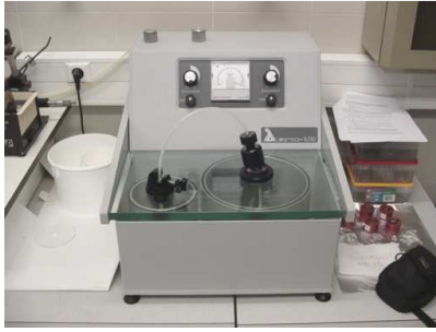
Figure 11. Vacuum chamber (left) where the samples are kept for 24 h before they are impregnated with epoxy resin and samples after the impregnation (right)
