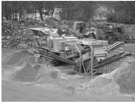
Figure 2. Mobile plant composed by a crusher and a vibrating screen
