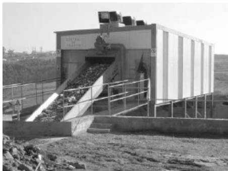
Figure 2. Separating belt feed at TRIANOVO recycling plant
