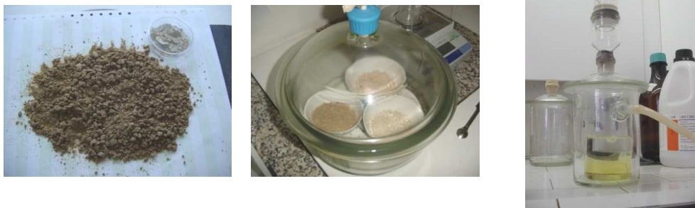
Figure 5. Disintegration of the rendering sample (left), stabilization of the dried samples (centre) and decantation of the insoluble residue fraction obtained through acid
