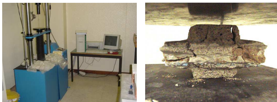
Figure 14. Equipment and test samples (left) and coating sample after failure (right).
