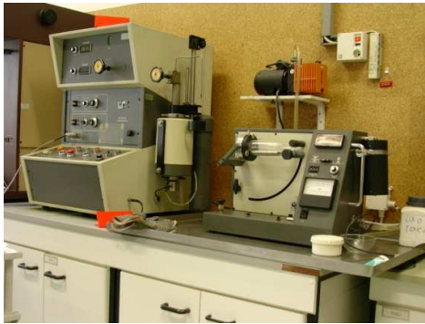
Figure 8. AUTOSCAN60 equipment (left) and filling apparatus (right)
