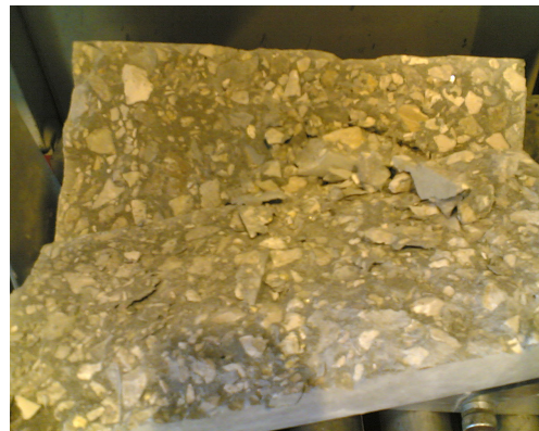
Figure 5: Failure surface of a specimen through its centre
