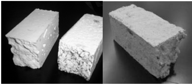
Figure 1 – Gypsum plasters with cellulose fibres, granulated cork and tyre fibres
