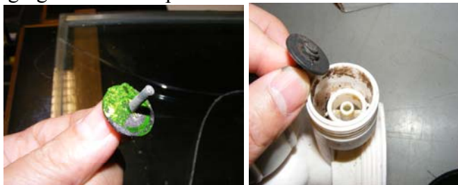
Figure 18 and 19 Anti-siphon rubber valve disc was found stained at valve seat side Performance test of a bottle U-trap found in the debris of renovation dumping site
