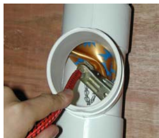
Figure 12 Insertion of rubber ball into the vent stack for sectioning the tested floors
