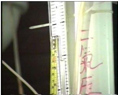
Figure 15 L A 38mm w.g. test pressure can be maintained for 3 minutes after the air pump was switched off.
