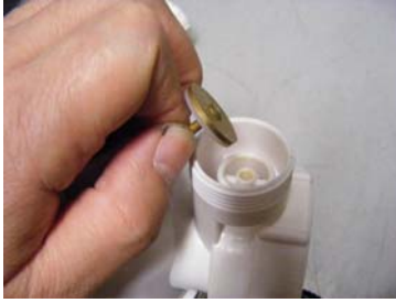
Figure 20 A functional anti-siphon copper valve disc with gasket lining Performance test of a good bottle U-trap used in the uPVC pipe test
