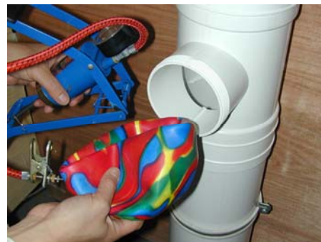
Fig 2 Insertion of rubber ball into the vent Stack for sectioning the tested floors
