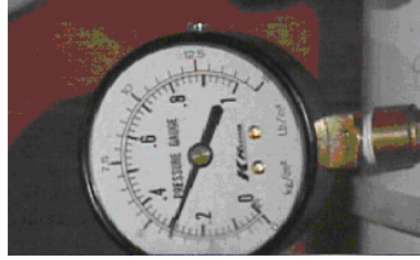
Figure 7 After repairing all the air leak points, the highest reachable test pressure was only 0.3 bar (30kPa). Just after 0.3 bar, all the sectioning rubber balls were suddenly forced out of their position under the great air pressure (0.3 bar)
