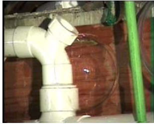
Figure 14 The big soap bubble was formed under a testing air pressure of 38mm w.g. on a loose cleaning eye cap. This showed that the low pressure air could also identify air leak defects
