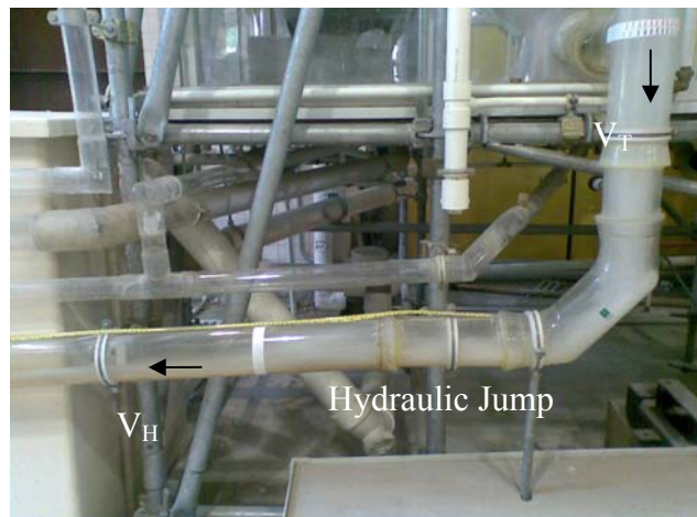
Figure 2 – Hydraulic jump occurs when vertical and horizontal speeds are different, trapping air at the bend
