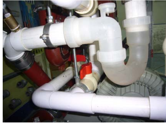
Figure 13 – 'P' trap under positive pressure
