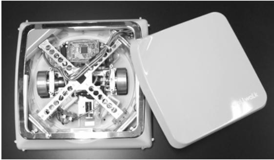
Fig. 6 Prototyped window cleaning robot
