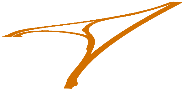
Figure 3: The 3-D surface model created for the tests. The model was designed by Terra Street CAD application and used directly to control the blade of grader.
