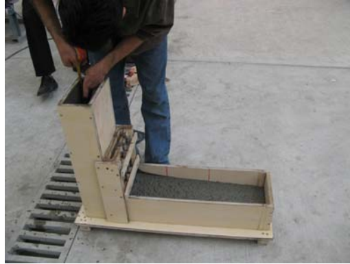
Figure 6. Schematic illustration of L-box
