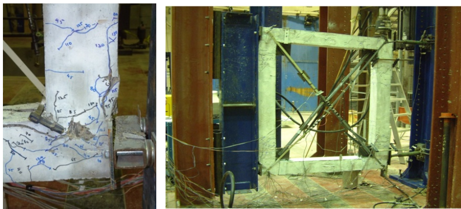
Figure 4. Test set-up and pattern of cracking in the moment frame (F1)
