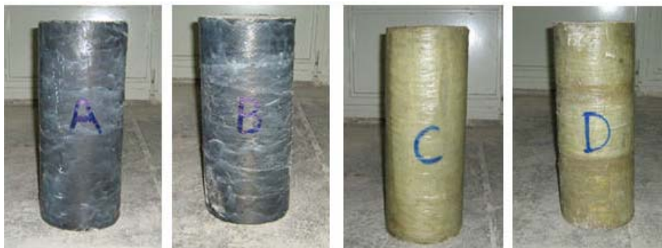
Figure 2. Sample A&B confined with CFRP- C&D confined with GFRP
