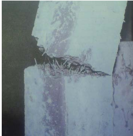
Figure 9. Vertical view of the failed specimen with 5% of fibers
