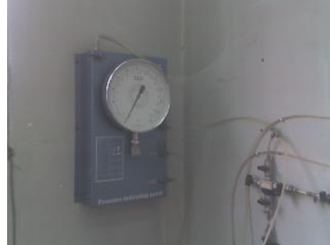
Figure 2.4. Measurement gauge for confining and injection pressure with continuous control
