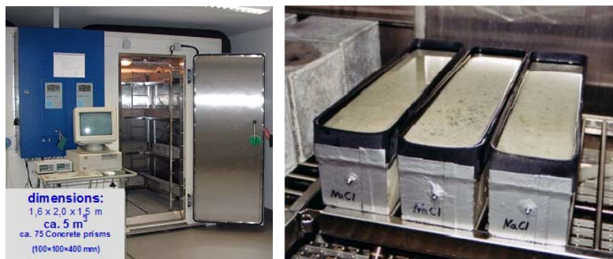
Figure 3. Climate simulation chamber and concrete prisms with NaCl solution (0.6 mol/l)
