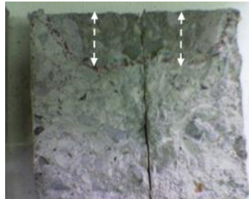
Figure 9. Water penetration depth in the specimen containing PN gel
