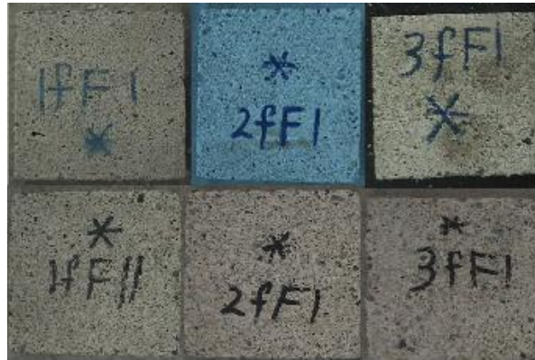
Figure 7. Mortar plates after 2 and 6 months immersion in sulfuric acid solution with pH of 2.0
