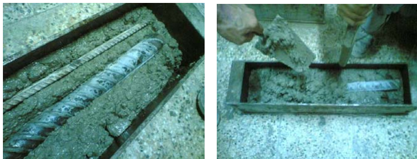
Figure 1. Rebars placement in beams
