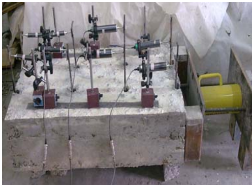
Figure 3. Lateral view of pullout specimen
