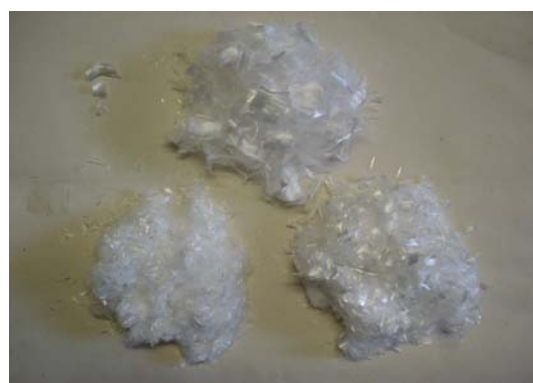
Figure 3. Sample of polypropylene fibers (6, 12 and 19 mm)
