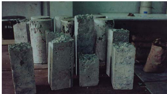
Figure 6. prismatic specimens after failure
