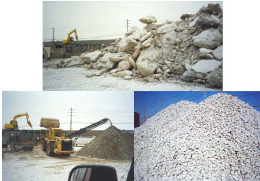
Figure 4. Concrete to be Recycled, Concrete Crushing, Processed Concrete
