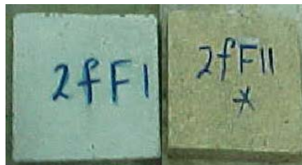
Figure 5. Mortar plates of C_2 mixture after 1 week immersion in sulfuric acid solutions with pH of 1.0 and 2.0
