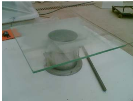
Figure 4. Cylindrical metal measure with Tamping Rod and piece of plate glass
