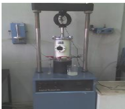
Figure 2.1. General view of tri axial apparatus
