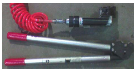
Figure 1. strapping mechanism and devices for retrofit of rc members
