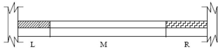
Figure 1. Beams subdivision along their lengths.
