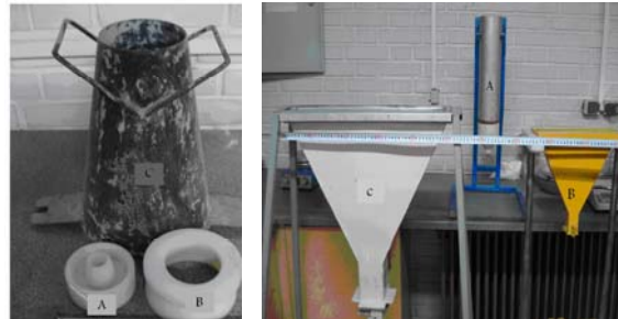
Figure 1. Slump cones and Funnels used for testing (A) paste, (B) mortar, and (C) concrete
