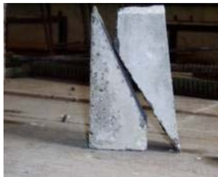
Figure 1. Concrete samples prepared based on BS 6319: Part 4
