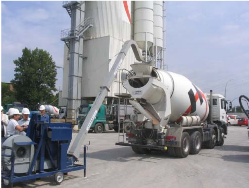
Figure 6. Blow in of the steel fibres into the mixing vehicle
