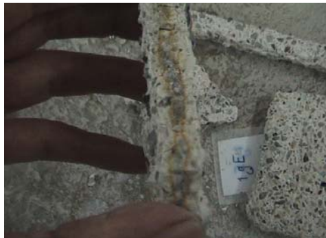
Figure 10. Tan layer formation between corroded and uncorroded concrete in mixture
