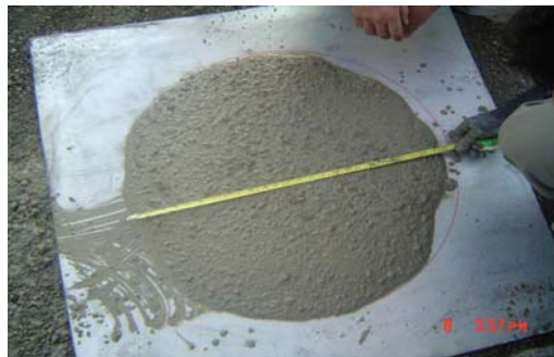
Figure 3. T-50 tests apparatus
