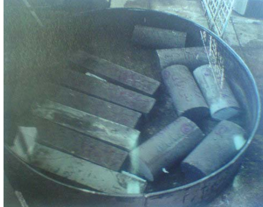
Figure 1. specimens in water basin in laboratory temperature.
