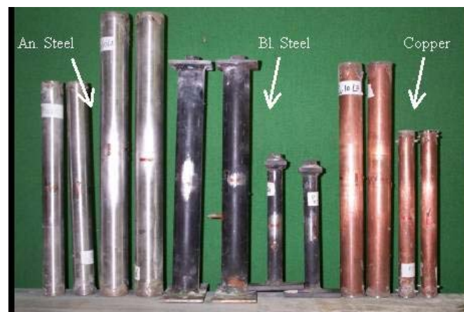
Figure 2. Metal tubes filled with EG
