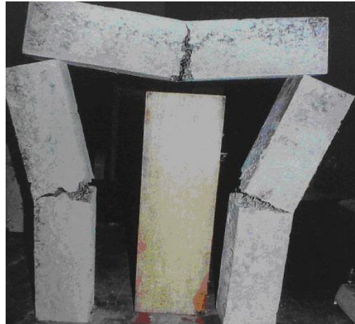
Figure 7. specimens with 5% of fibers after failure
