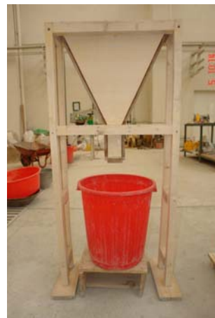
Figure 5. Schematic illustration of V-funnel
