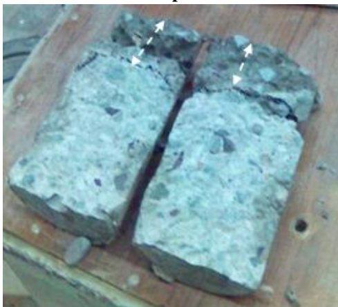
Figure 10. Water penetration depth in the specimen containing PN liquid
