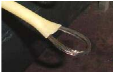
Figure 5. SMA cable restrainer with the effective length of 1.16 m used as a retrofitting device
