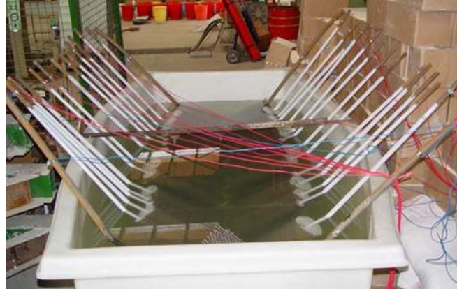
Figure 1. Accelerated corrosion program [7]
