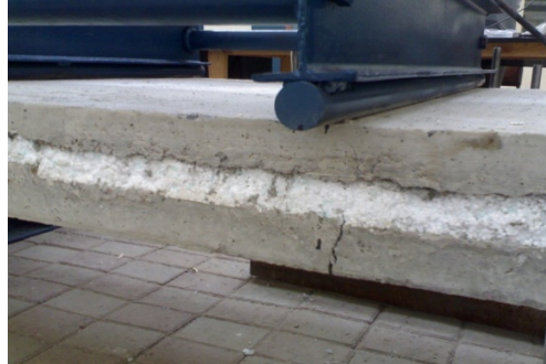
Figure 5. Cracking pattern in two layer panel in flexure
