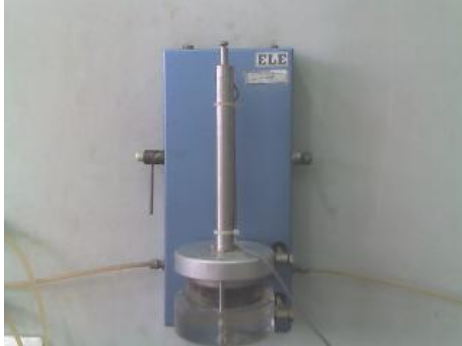
Figure 2.3. Digital sensor for water input measurement in to the specimen(volume change)
