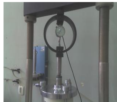
Figure 2.2. Digital sensor for axial force
