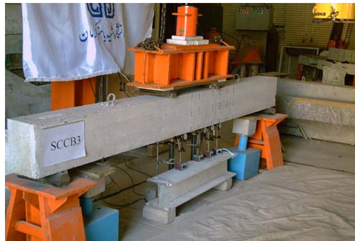
Figure 9. Typical test set up for loading arrangement [9]
