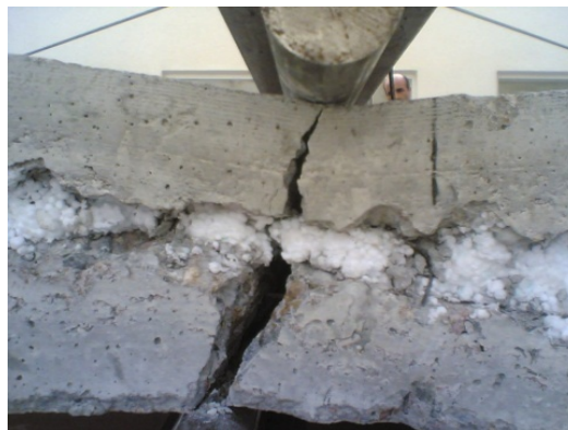
Figure 7. Cracking pattern for two-layer panel in shear test
