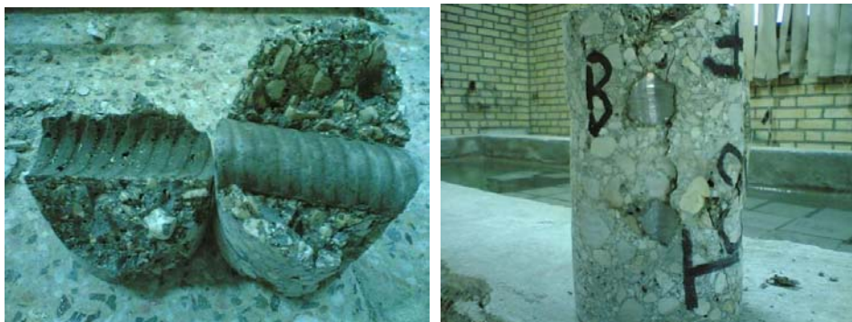
Figure 4. Separation of rebars after compression test of cores
