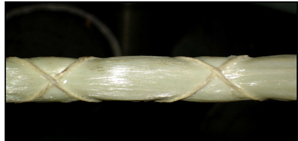
Fig. 2. GFRP bar with two strings (Samples 21 to 26)
