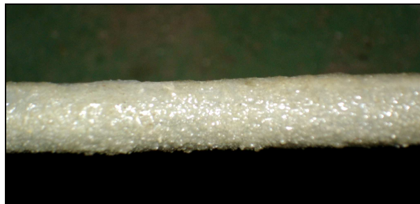
Fig. 3. GFRP bar coated with sand (samples 31 to 36)
