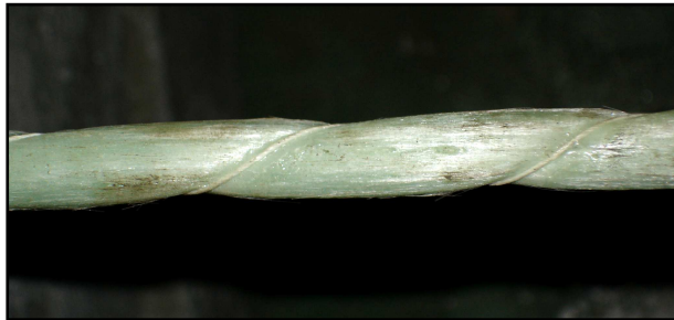
Fig. 1. GFRP bar with one string (Samples 11 to 16)
