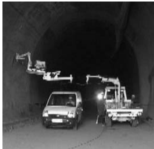
Figure 8. RATIM System Tested Outdoors
