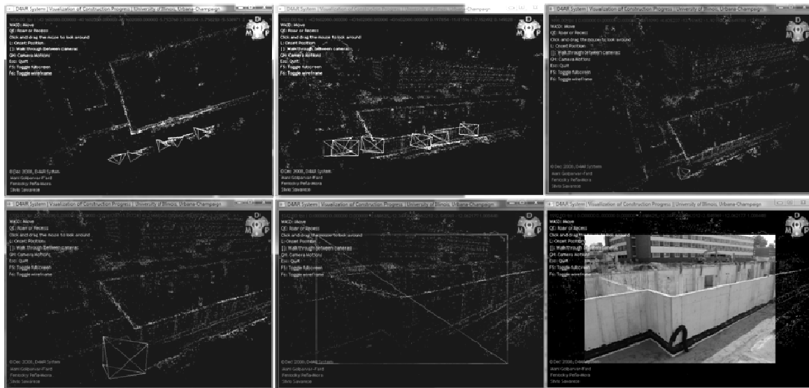
Figure 6. Sparsely reconstructed scene of Residence Hall using 52 images with 25% of image qualities. Six camera frusta are rendered and geo-registered.
