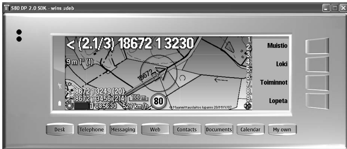
Figure 9. Classification of road condition is shown in real time on mobile phone screen. The decimal number on top of left corner shows road condition.
