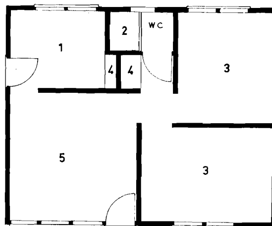
Fig. 7. Barbados Housing Authority (1957). One-storey “four-square” house, Type 100. Floor area 37.1 m 2 . 1 kitchen, 2 shower, 3 bedroom, 4 cupboard, 5 living-room.
