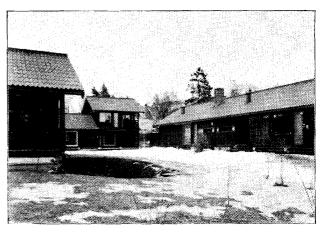
The houses have an internal load-bearing post and beam system which provides non load-bearing exterior walls. This system makes Tunhus very flexible in terms of interior planning and construction. Today the system has been taken over by a housing company.
