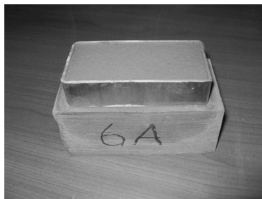
Figure 2 Mortar placed in the frame on the top of the fired clay brick. Photo was taken 120 min after placing and the front of absorbed water is visible on the front side of the brick.
