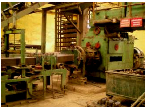
Figures 5 - 7 Fired clay brick manufacturing processes (left); cutting and transportation of cut waste (right-top) and brick extruded from die and shelved bricks for being transported to drying unit (right-bottom)
