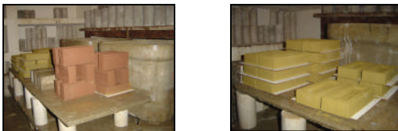
Figure 3 Curing of the pressed bricks (Souza Filho, 2005).
