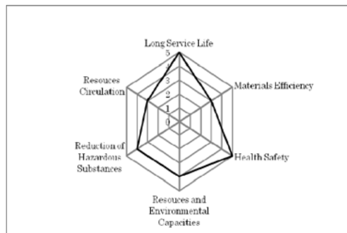
Figure 5 Visualization of ecobalance evaluation by radar chart of GFRC
