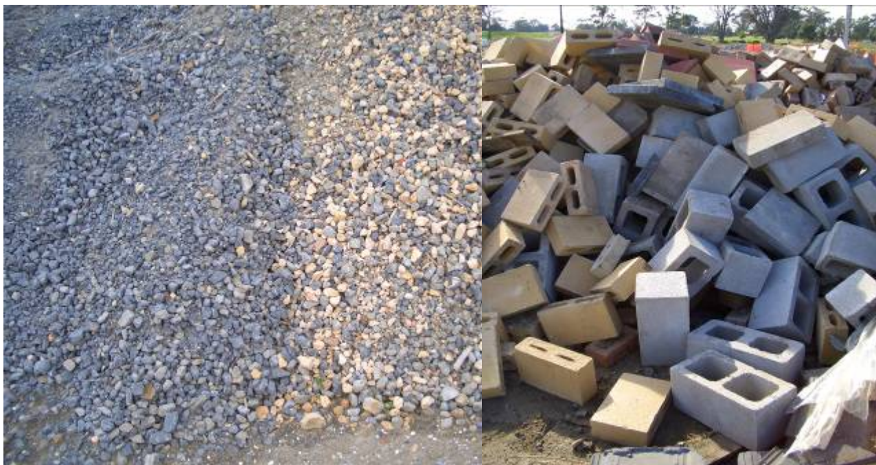
Figure 6 Left: Crushed tile and brick aggregate Right Concrete bricks which caused more wear and tear on the grinder.
