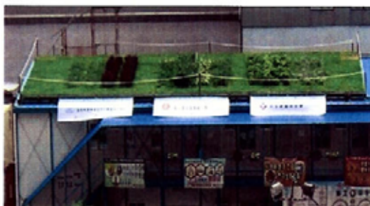
Figure 3 Green Panels have been set up at the roof of the construction site to work out design optimization.
