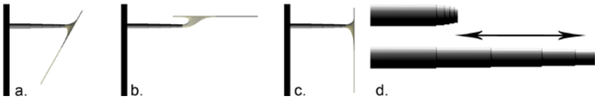
Figure 6 The shading sheets inclination and their support elongation. (a.-c.) showing different inclinations of the sheet connected to the support member by an elastic membrane. (d) the support tubular member elongation.
