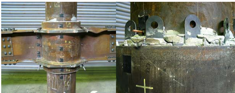
(a) The local buckling of the beam (J1)
