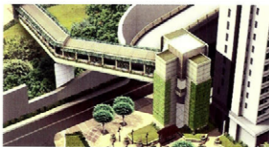
Figure 4 Vertical green panels designed to clad onto the external wall and laid flat on roofs of lift tower.
