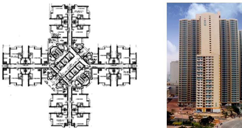
Figure 1 Typical floor plan (left) and the appearance (right) of the New Harmony Block (Option 2)
