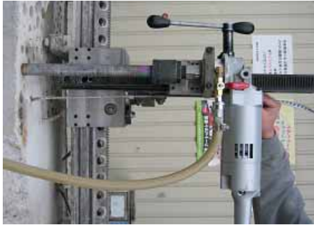
The motor is attached to the angle vertical to the drill axis.
