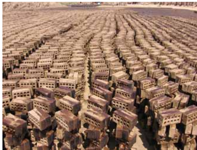
Figure 9, bricks are drying under sun
