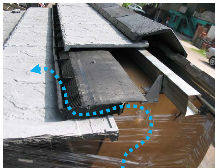
Figure 12 Roof construction mock up: to test the ventilation device effectiveness.
