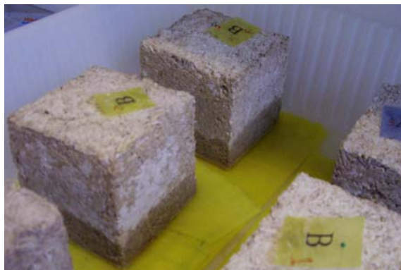
Figure 4 Water sorption test, specimens from mix B.
