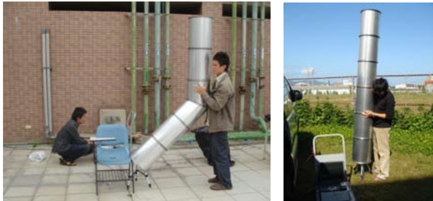
Figure 6 Photographs of field measurements of the daylight pipes.
