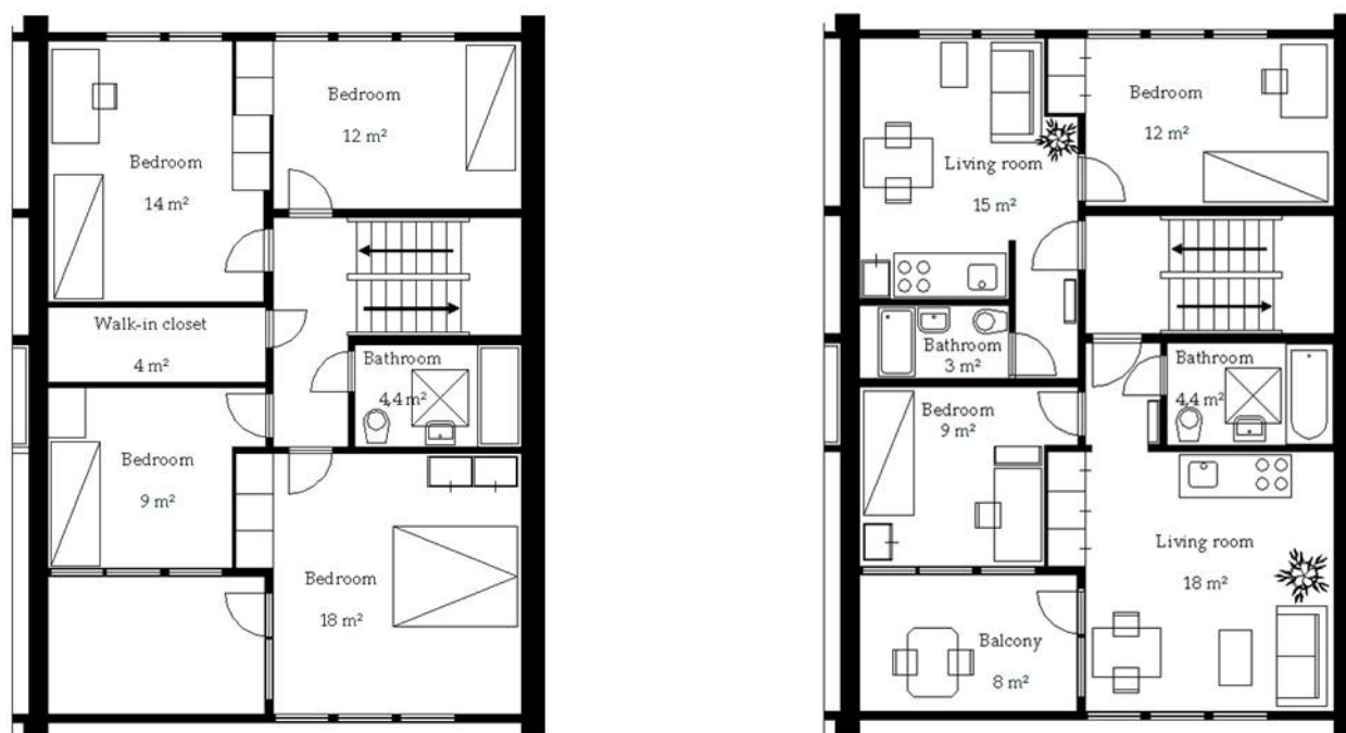
Figure 5 First floor; left the existing situation, right the proposed new situation.
