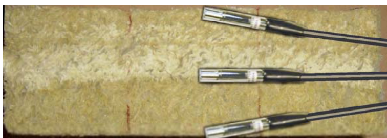
Figure 3 Temperature and humidity sensors placed in material specimen.
