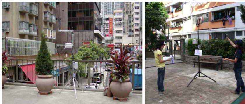
Figure 3 Photographs showing fieldwork equipment and measurement on site using fixed mini-weather station and mobile anemometer
