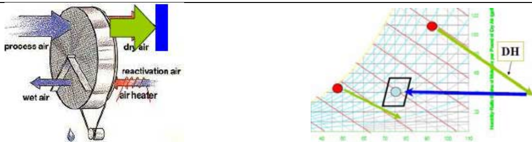
Figure 7: Gas Fired Desiccant dehumidifier and psychrometric chart
