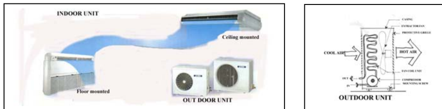
Figure 4 A typical split-system air-conditioning system for both high-rise and low rise residential units
