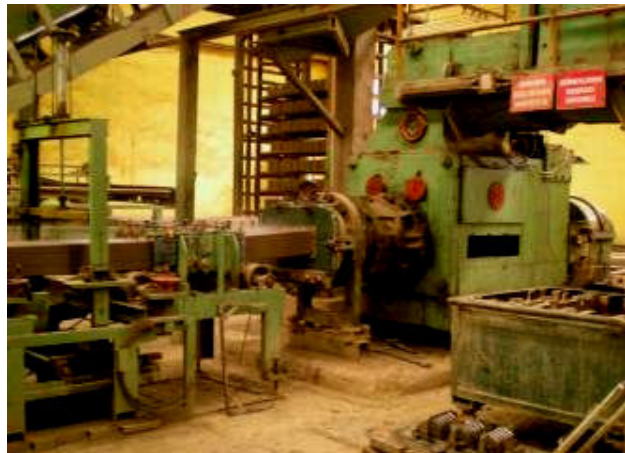
Figures 5 - 7 Fired clay brick manufacturing processes (left); cutting and transportation of cut waste (right-top) and brick extruded from die and shelved bricks for being transported to drying unit (right-bottom)
