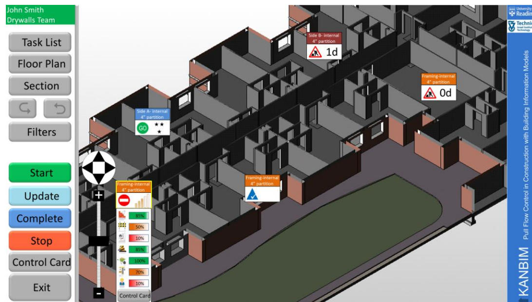
Figure 4: Trade crew leader work status and reporting interface showing a crew's tasks. The crew leader can ask the system to show neighbouring tasks for a complete picture of the overall work
