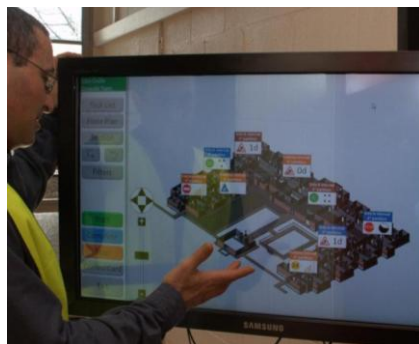
Figure 5: Work face specialized model interface on a 40" touch-screen mounted on a mobile trolley. The system identifies crew leaders (by RFID reader or by entry of a unique ID code) and delivers specifically tailored information concerning their tasks.
