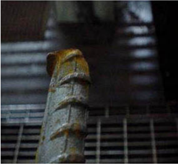
PICTURE ONE: DAGS ON ENDS OF REINFORCEMENT BARS AFTER PROCESSING
