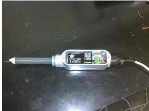
Figure 1 - Omnidirectional wind speed transmitter by “heated mass”
