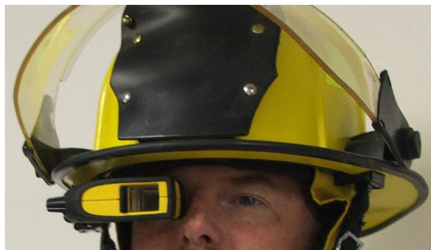
Figure 4. Head Mounted Display in combination with a helmet [©Liteye Systems, Inc.].
