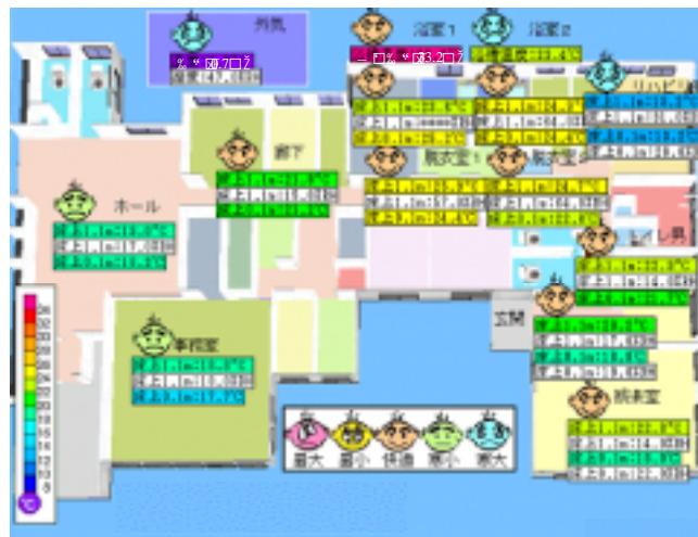
Fig.4 Temperature and Humidity Display on Monitor of Personal Computer
