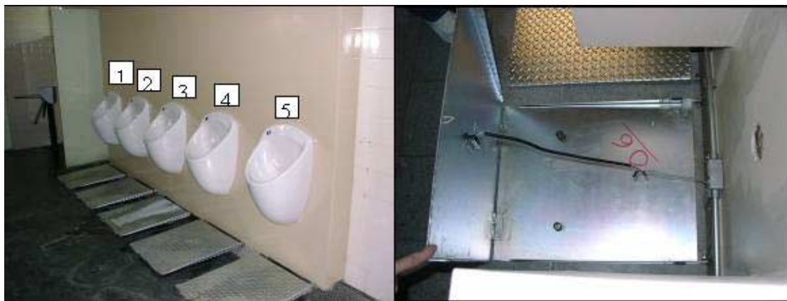
Figure 4 – Measurement system - platforms with sensors
