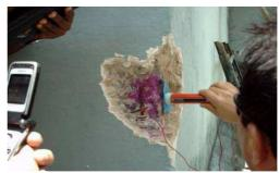
**Figure 6.** Application of the positive electrode on the face of wet concrete and connected to negative reinforcement in the column P1.
