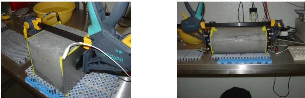
Figure 1. Test layout of the two-plate electrode method for ER measurements the ER on cubes (left) and cylinders (right).
