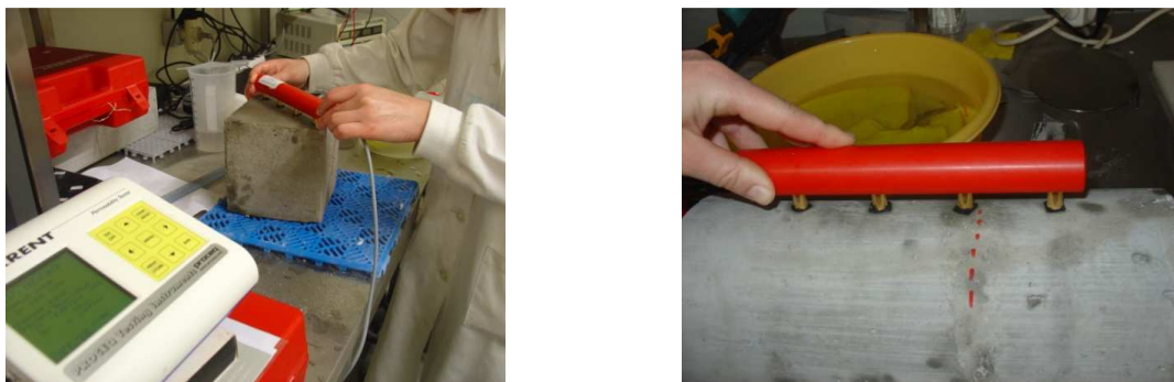
Figure 2. Performing four-point electrode method ER measurements on cubic (left) and cylindrical (right) specimens.
