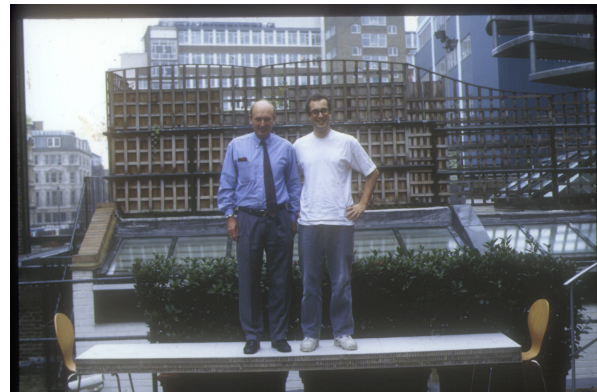
Figure 1: Card beam under two man test load!
