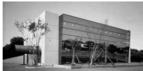
Main Building of Obayashi Corporation, Japan This building was completed in 1982 and represents 98 energy conservation techniques including double skin, solar heating and cooling, different thermal storage systems, daylighting strategies, photovoltaic panels and rainwater utilization. Building cost are about 20% higher whereas the operating energy is only 27% compared to a common reference building design in this country.
