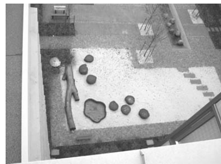
Figure 6 White gravel used for light reflection. Dark figures are reused tree trunks from site.
