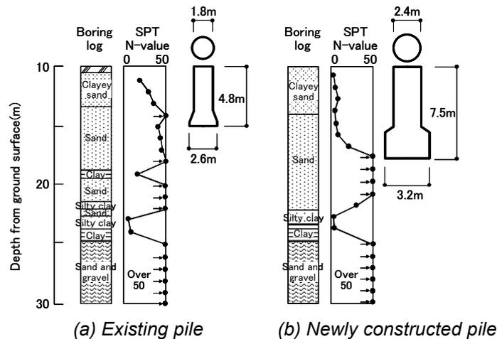
Figure 3 Soil conditions and schematics of load-tested piles [4] (Case 1)
