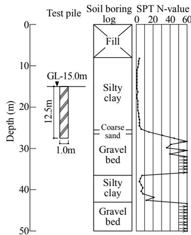
Figure 8 Test pile and summary of soil investigation [7] (Case 2; main investigation)
