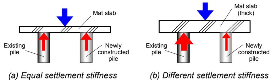
Figure 4 Schematic diagram of design of mat slab according to difference in settlement stiffness between existing pile and newly constructed pile [3]
