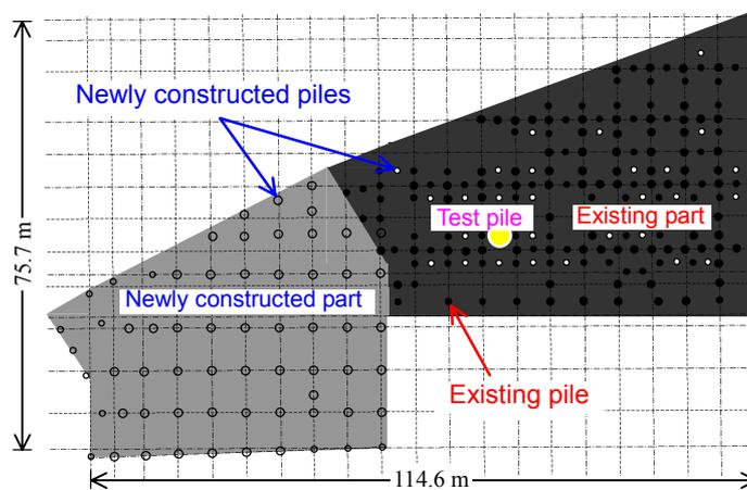
Figure 7 Layout of existing and newly constructed piles [6] (Case 2)
