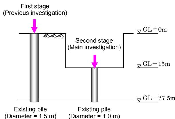
Figure 9 Sequence of operation of two rapid loading tests of existing piles [3] (Case 2)
