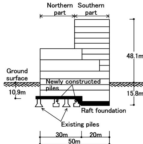
Figure 1 Schematic of new building [4] (Case 1)
