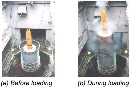
Photograph 4 Scenes of rapid pile loading test (Case 2; main investigation)
