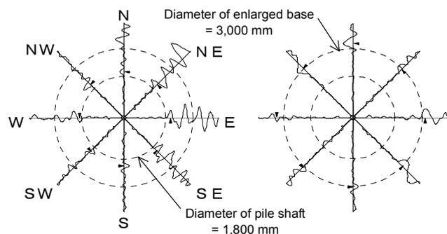
(a) Pile Shaft (b) Enlarged base
