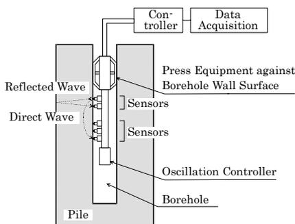
Figure 11 Schematic of borehole sonar
