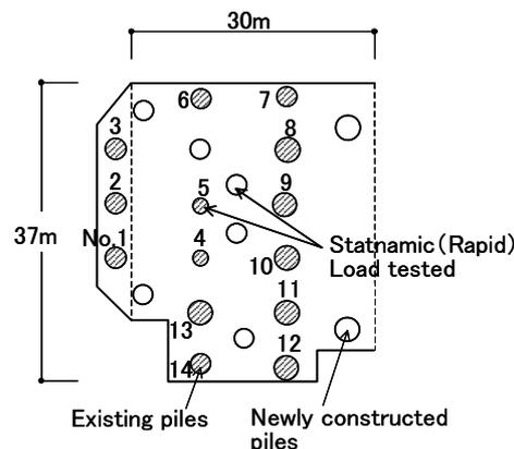
Figure 2 Layout of existing and newly constructed piles [4] (Case 1)
