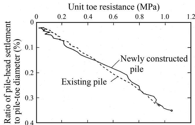
Figure 5 Relationship between unit toe resistance and ratio of pile-head settlement to toe diameter [4] (Case 1)
