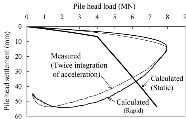
Figure 10 Estimated static load-settlement curve at pile head [3] (Case 2; main investigation)
