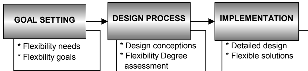
Figure2. A construction process that takes building flexibility into account consists of three distinct phases.
