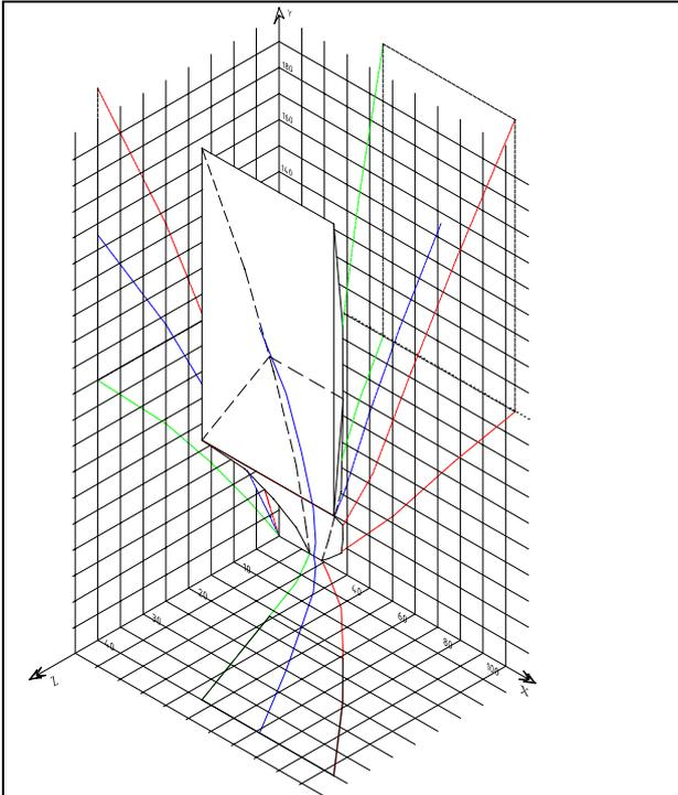
Fig.1. General solution for stochastic process of underground structure behaviour in the course of operation:  $x$  – term of operation  $T$ , years (10-year intervals);  $y$  – index of bearing capacity margin loss;  $z$  – reinforcement corrosion  $K_c$ , % (5% intervals)
