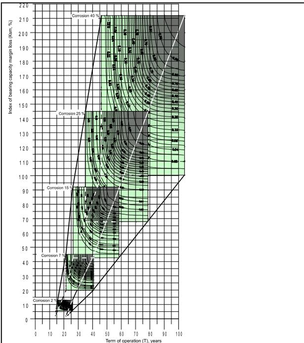
Fig.2. Isofields of equiprobability by “no-failure” for random values of output parameter  $K_{sm}(t)$
