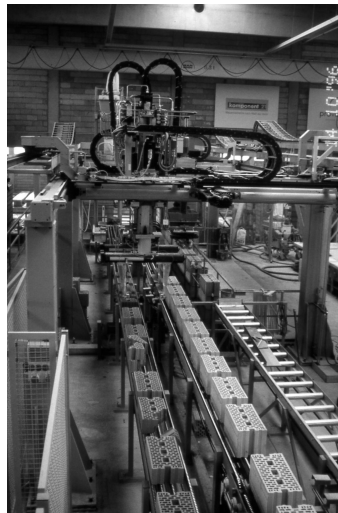
Figure 2 shows a robot for customized masonry prefabrication
