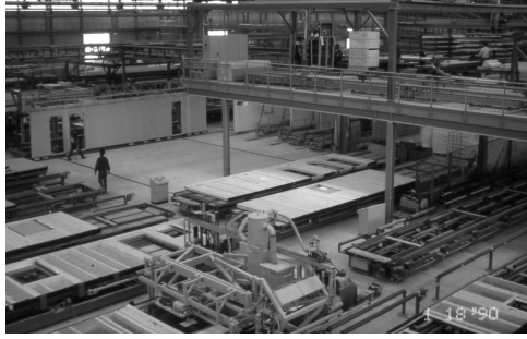
Figure 3 shows a robot for customized wooden panel production
