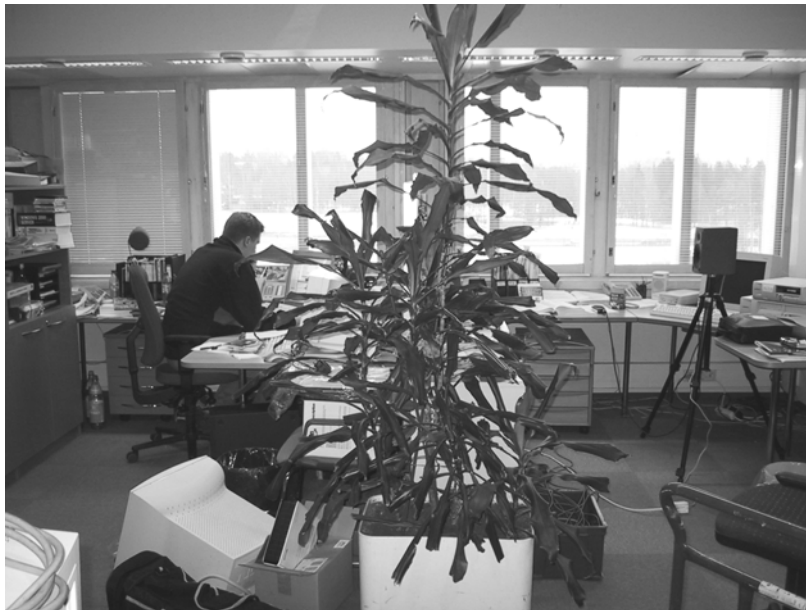
Figure 2. Measurement of STI between two neighboring workstations. Speaker is placed on one workstation and the measurement is carried out in the other. Workers are absent during the measurement.
