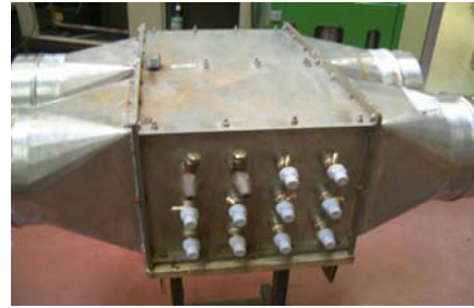
Heat Pipes recovery system HP.
