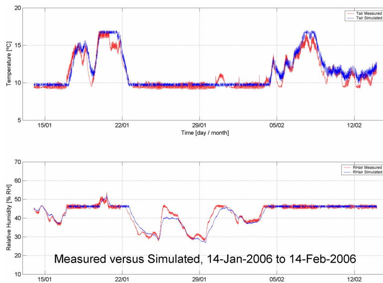
Figure 6. Simulation results of temperature and RH in the humidistatically heated room over the period from January 14th to February 14th 2006.
