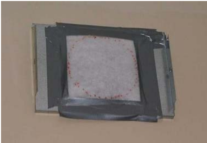
Figure 4. The polypropylene filter cloth fixed at the supply air terminal device.
