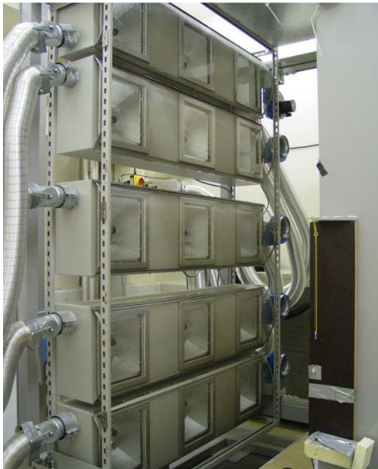
Fig. 1 Large Scale Solar Simulator, showing lamp array.
