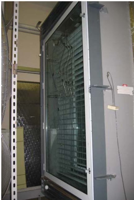
Fig 2 The Tested Double Skin façade: a) outer door closed; b) outer door open
