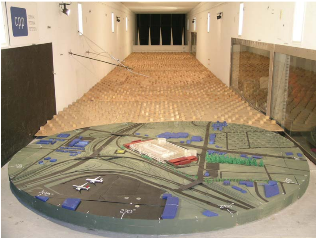
Figure 4. Photo of parking garage pressure model in the boundary layer wind tunnel.
