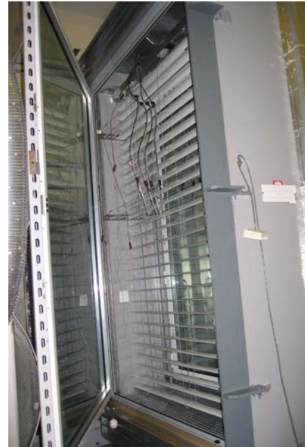
Fig 2 The Tested Double Skin façade: a) outer door closed; b) outer door open
