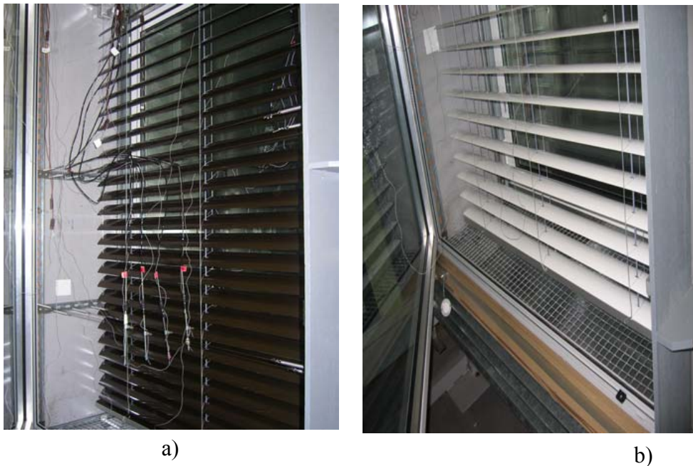
Fig. 3 The blinds installed in the façade cavity: (a) dark brown ('spartbrown'); (b) white
