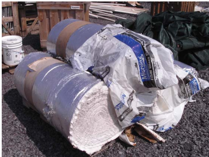
Figure 2. Water-damaged fiberglass duct wrap stored outdoors.
