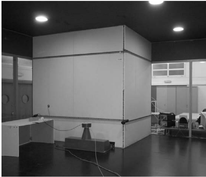
Figure 2. Subchamber reproducing a bathroom. View from the interior of the chamber.
