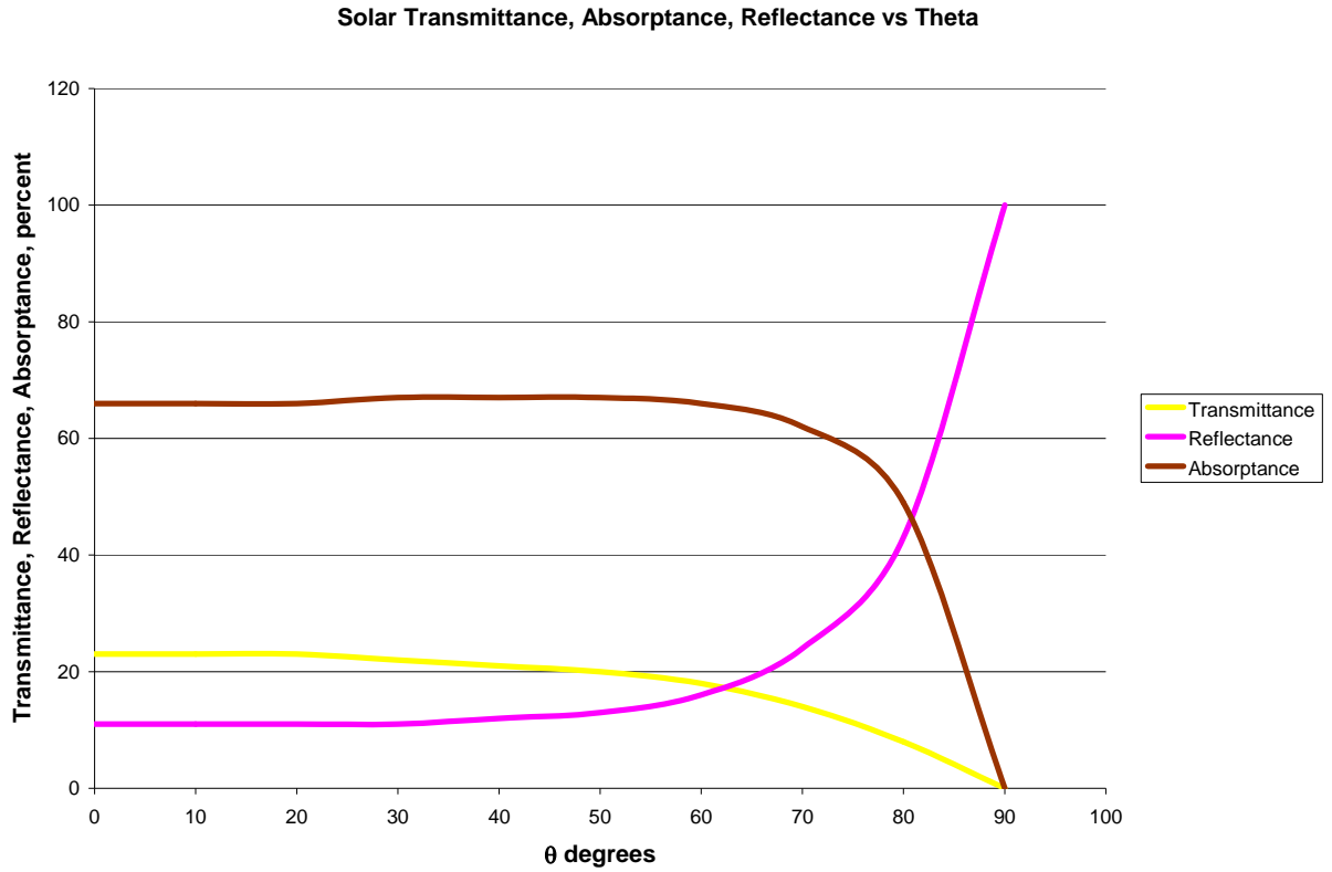
Figure 2. Optical properties of heat absorbing glass.
