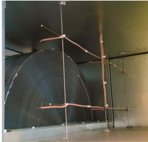
Figure 4. Picture of a thermocouple grid in front of the rotary heat recovery unit.
