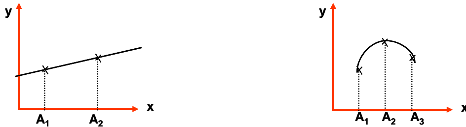
Figure 1. Choice of number of levels: 2 levels on the left (linear evolution), 3 levels at least on the right (non linear evolution)
