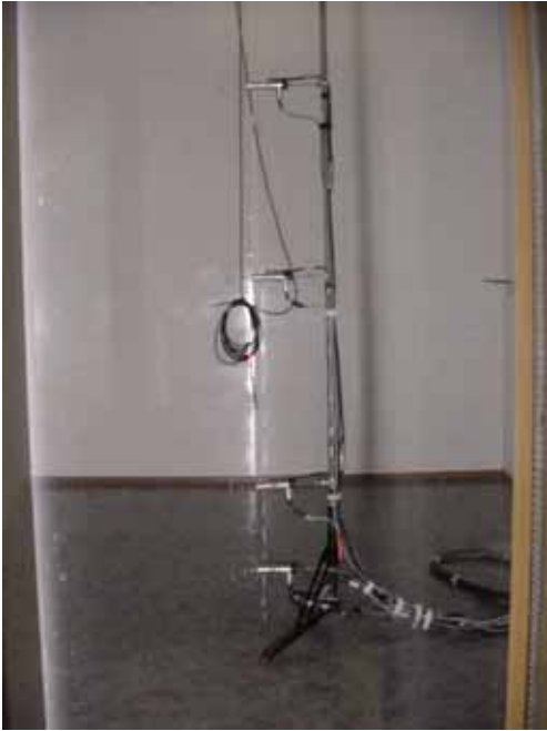
Figure 2. Velocity and temperature measurement equipment
