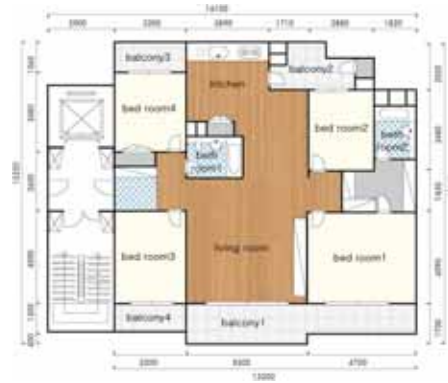
Figure 2. A typical floor plan of a unit (floor area of 160 m 2 ) in the selected apartment complex.
