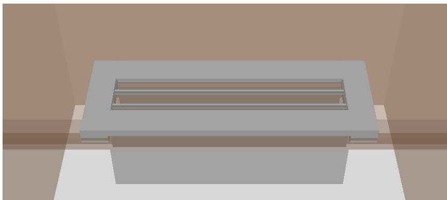
Figure 2: Horizontal desk grille geometry
