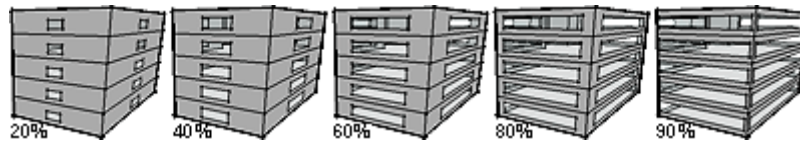
Figure 3 - Values for characterising facade glazing ratio.
