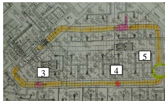
Figure 3. Supply air duct and measurement location
