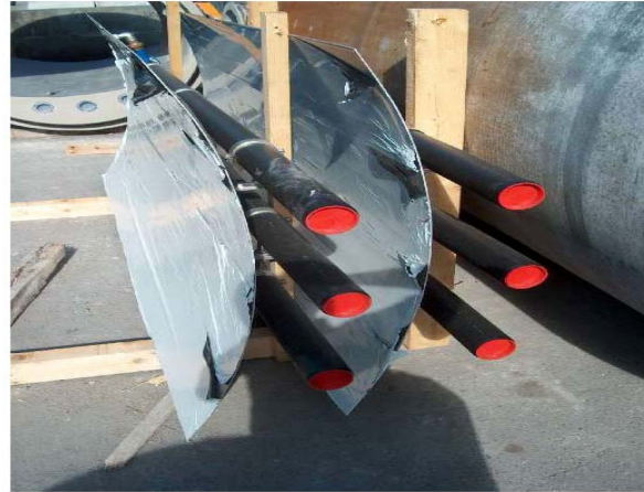
preassembled Rabtherm® - heat exchanger elements
