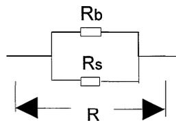
**Figure 2 Resistance relation between buffer and sample tested**
