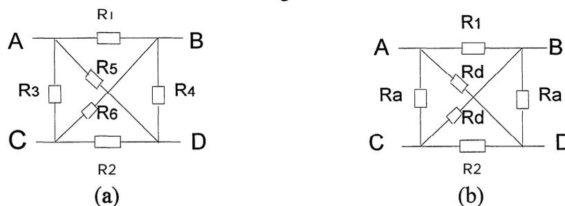
**Figure 4 (a) Equivalent circuit diagram of GD1 sensor
