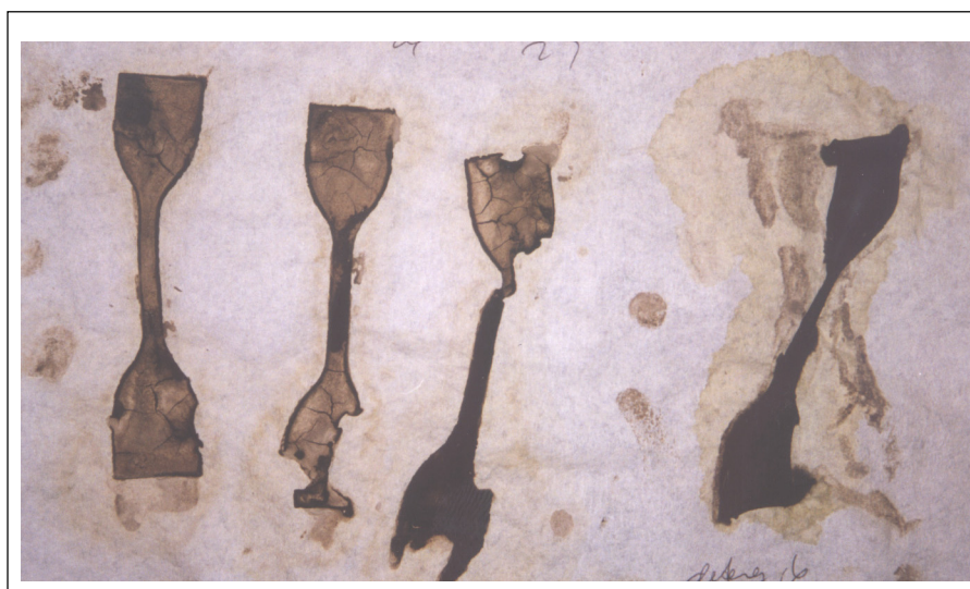
Figure 7. Tensile test specimens that failed before they could be tested
