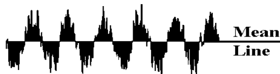
Figure 1. Mean line of a surface profile
