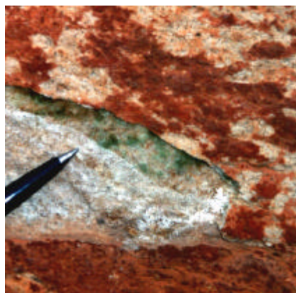
Fig. 16. Spalling soapstone, showing green growth of (mainly) cyanobacteria deeper than the whitened spalled layer. The red coloration is patina.
