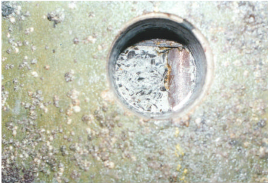
Fig 3. Surface Corrosion Observed on the Steel Bars at A Core Location in Fig 2
