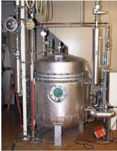
Figure 3: Pressure vessel for ageing in oxygen-enriched water at elevated temperature and pressure
