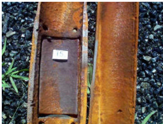
Figure 8. Close up of sample 15 from building 16 showing inspection cover and small through-wall defect on bottom right hand photograph.
