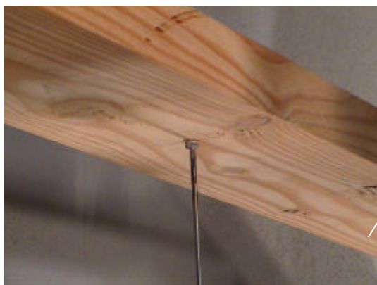
Figure 4: Transducer attached to specimen
