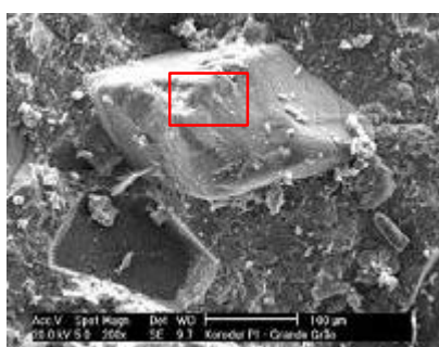
Figure 9: SEM image of the mortar sample of the Test core P1 (200X)
