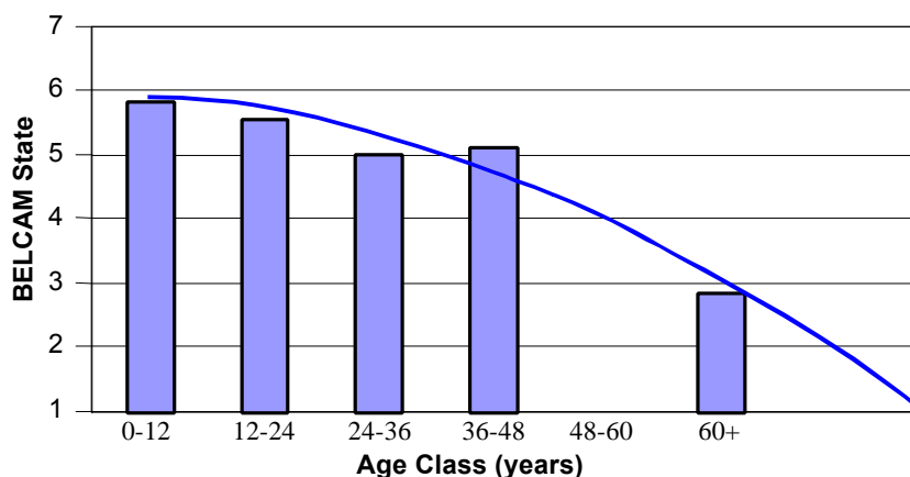
Figure 11. Average condition curve of built-up roofing membrane
