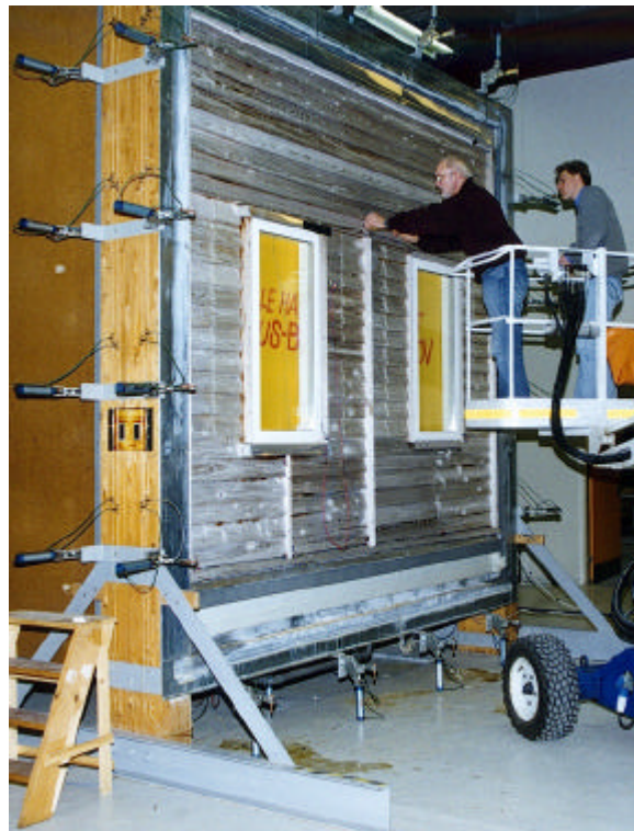
Figure 7: Example of full scale testing of a wooden facade including windows.
