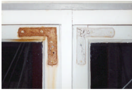
Figure 3: Example of accelerated testing of different paint systems used on window sashes.
