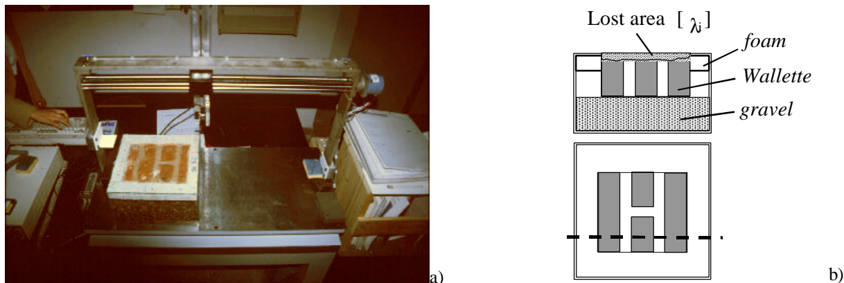
Figure 2. a) Laser profilometer device and b) scheme of the measurements
