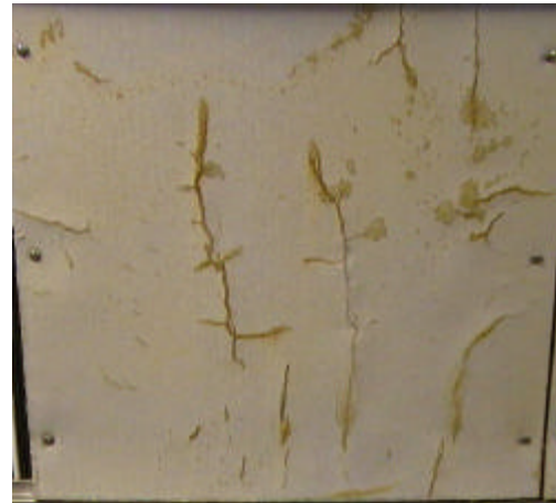
Figure 4: 8 mm fibre-reinforced cement claddings for exterior use after 48 weeks in the climate carousel
