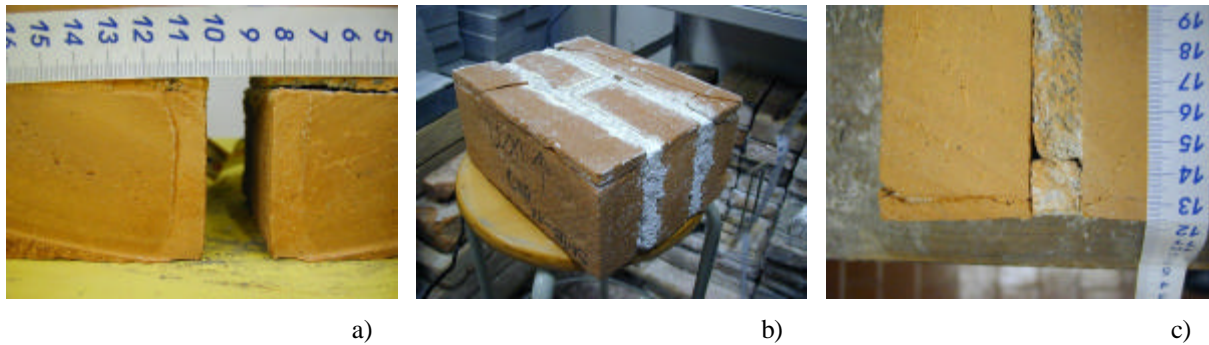
Figure 7. Softmud brick wallettes, particulars of the damages with WR: a) with 2.5% of \text{Na}_2\text{SO}_4 b) and c) with 2.5% of \text{Na}_2\text{SO}_4 in presence of Pointing
