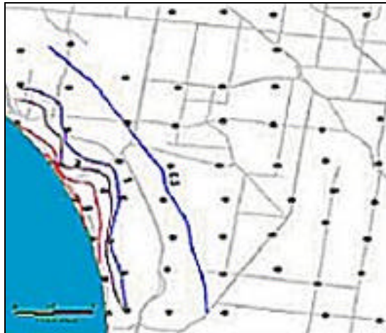
Figure 2. Estimated corrosion of galvanised steel based on distance from the coast (in \mu\text{m} per year).
