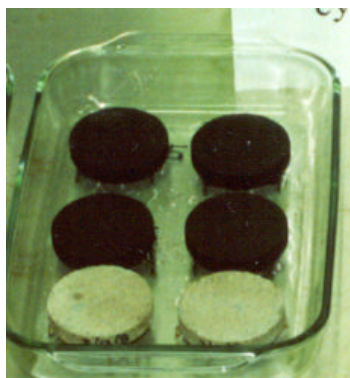
Figure 4. Colour Change of the Specimens subjected to Sulphuric Acid
