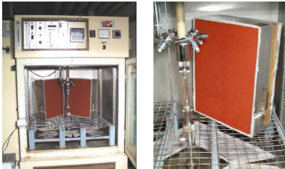
Figure 1. Pictures showing the environmental chamber with two wall specimens.
