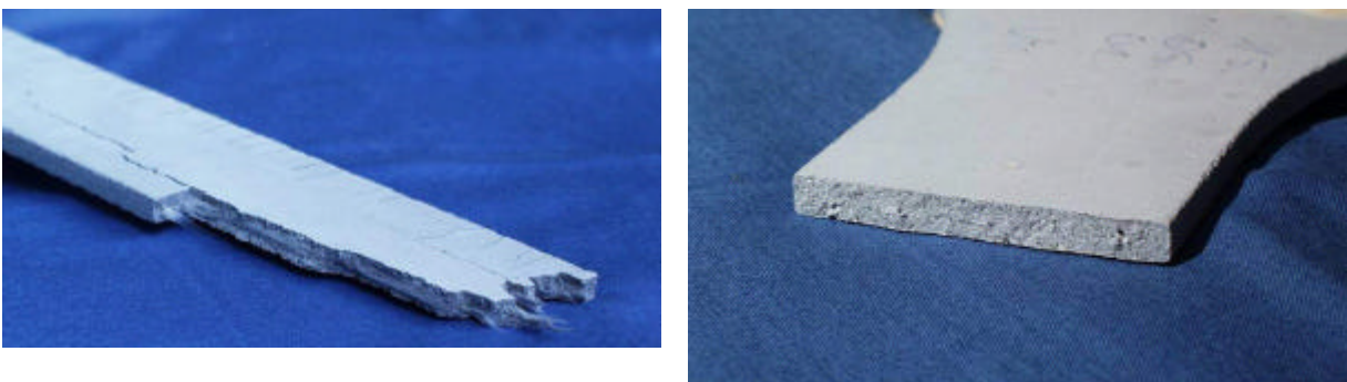
Figure 5. Failure of TSP samples after 28 days storage at 23 °C and 95 % r. h. (left) and after 28 days storage at 23 °C and 95 % r. h. and 7 days in water at 50 °C
