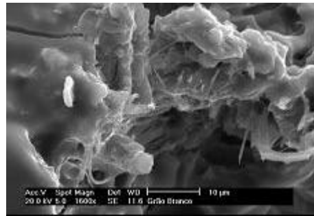
Figure 21: SEM image of the white grains with adhered mortar (1600X), zone c highlighted.
