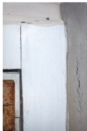
Figure 4: 8 mm fibre-reinforced cement claddings for exterior use after 48 weeks in the climate carousel
