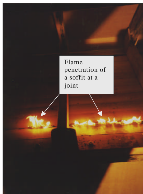
Figure 2. Flame penetration occurred through a T&G joint in a soffit constructed with nominal 1-inch (25 mm) boards. This view is from the interior of the attic/soffit area.
