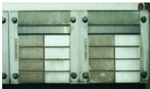
Photograph 5. Closing up of soiling behaviour, the left row in each block is non-treated tiles and the right row ; photocatalyst coating applied ones
