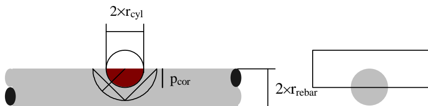
Figure 6. Improved model for localised corrosion attack
