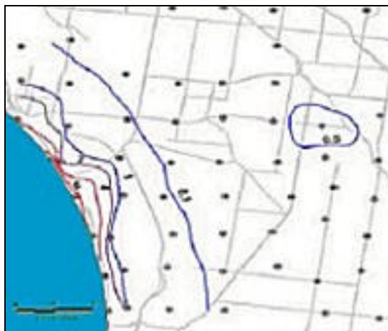
Figure 3. Estimated corrosion of galvanised steel based on distance from the coast and \text{SO}_2 level.
