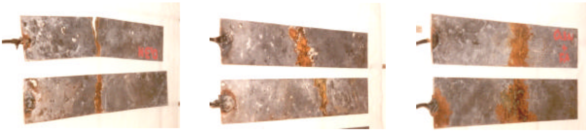
Figure 3. Visual observation of the corrosive attack on the bare steel plates embedded in reference natural-aggregate concrete N0.3 (left), in recycled-aggregate concrete R0.3 (middle) and high volume fly ash concrete N0.3F (right).
