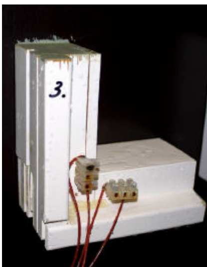
Figure 4: 8 mm fibre-reinforced cement claddings for exterior use after 48 weeks in the climate carousel
