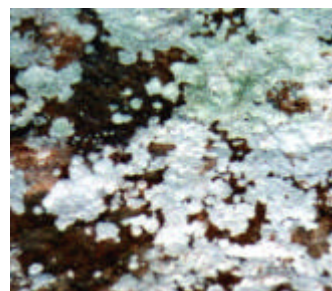
Fig. 13. Actinomycetes growing as a white layer on an internal wall at the Mayan site of Uxmal, Mexico.
