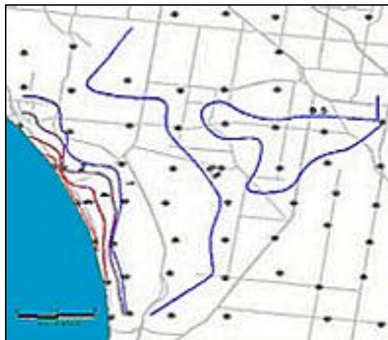
Figure 1. Observed corrosion of galvanised steel in south-east Melbourne, 1983-85 (in \mu\text{m} per year).
