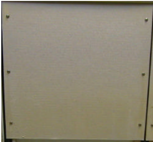
Figure 4: 8 mm fibre-reinforced cement claddings for exterior use after 48 weeks in the climate carousel
