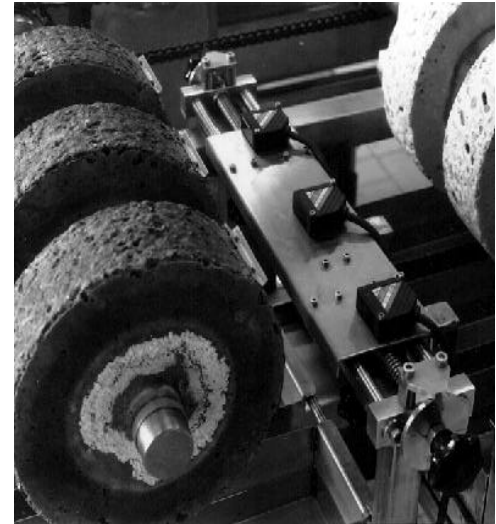
Fig. 1 Apparatus for accelerated degradation testing (TAP)
