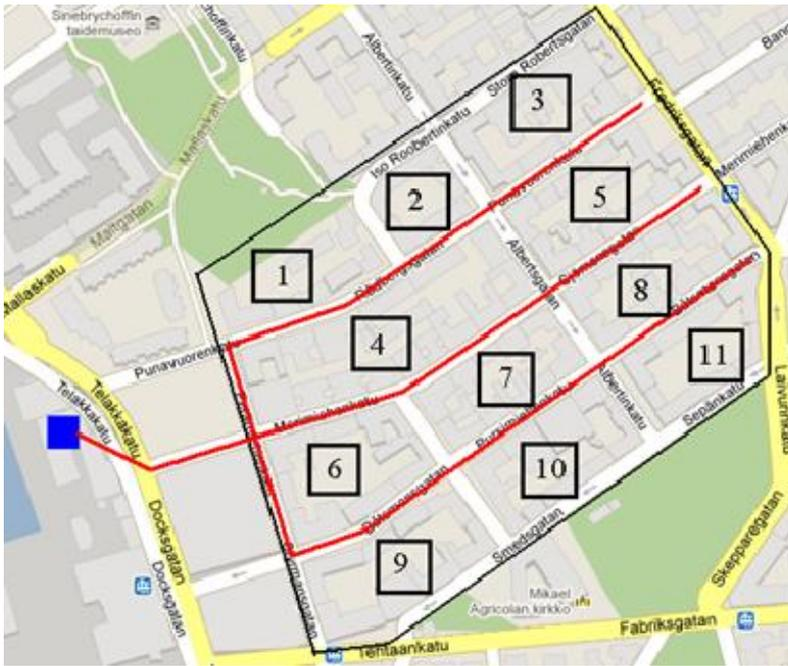
Fig. 1 Case-area in Punavuori. Numbers from 1 to 11 present the blocks covered by the pneumatic system. Red lines represent the modelled main pipe lines and the blue box the approximate placing of the waste terminal. Feeder pipe lines are not marked in the picture.
