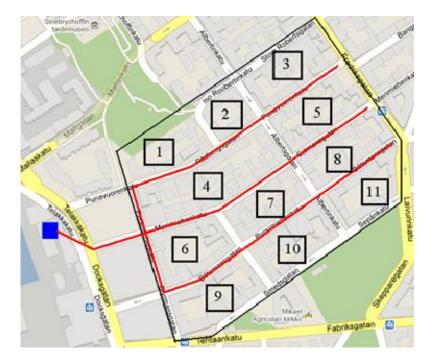
Fig. 1 Case-area in Punavuori. Numbers from 1 to 11 present the blocks covered by the pneumatic system. Red lines represent the modelled main pipe lines and the blue box the approximate placing of the waste terminal. Feeder pipe lines are not marked in the picture.
