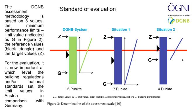
Assuming a lower minimum requirement (G) than in Germany, but the same target value (Z), this would result in a broader range for the assessment (see situation 1 in Fig. 2). In situation 2 building regulations such as e.g. the acoustic performance as in [ÖNORM B 8115-2] could be on a higher level than in Germany which leads to a very narrow range for the evaluation
