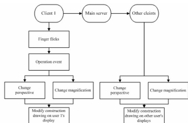
Fig. 2 Construction Drawing Sharing Module
