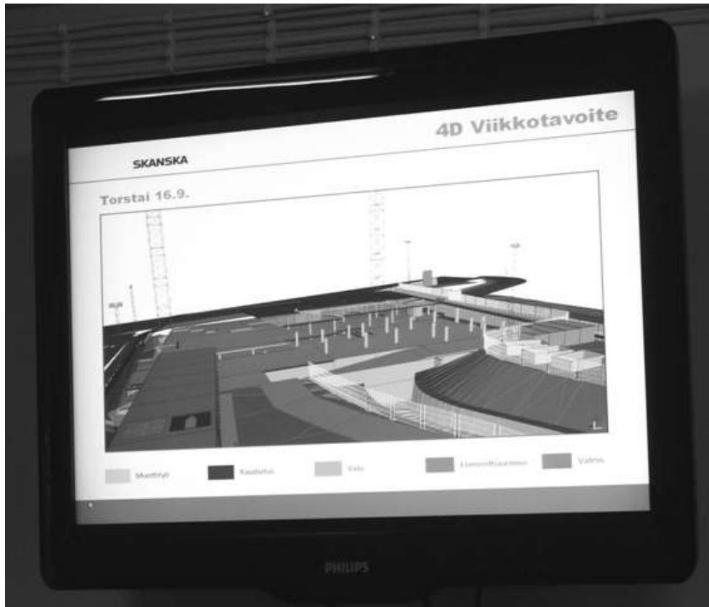
Picture 3: 3D site plan that is captured from the 4D model of the pilot building construction project. This is an example of part of slide show that run on the information displays.
