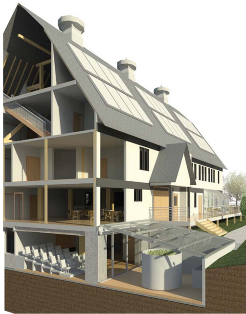
((C.) Michael Mandelman- Axonometric Section of Horse Barn, showing relationship between large lecture hall and Living Machine greenhouse.
