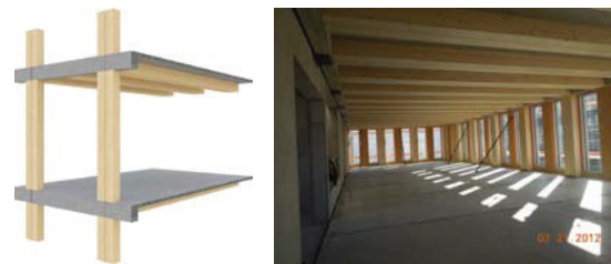
Fig.3: Posts and hybrid slabs (left). LCT ONE interior during construction (right)
