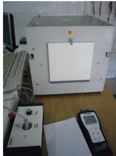
Fig. 2. Model house to study the heat conduction.
