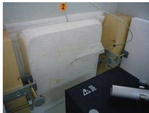
Fig.3. Interior of the model house: NiCr-Ni thermocouples and rubber-gypsum wall test piece
