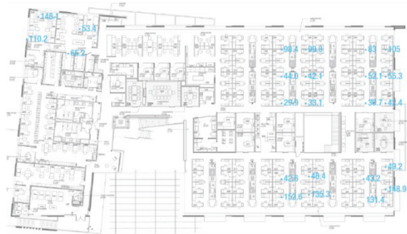
Figure 13: Illuminance level samplings on the second floor at HMC Concours
