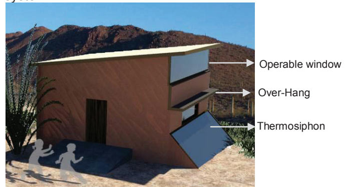
Figure 3: Proposed cabin design - rock bed
