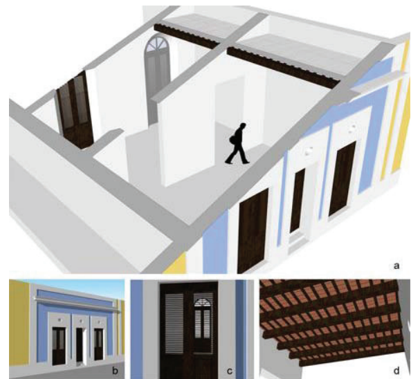
Fig. 10 Architectural details of a typical Spanish Colonial house in San Juan, Puerto Rico: a. Wall thickness and spatial relationship, b. main façade, c. doors with movable louvers, d. ceiling detail.
