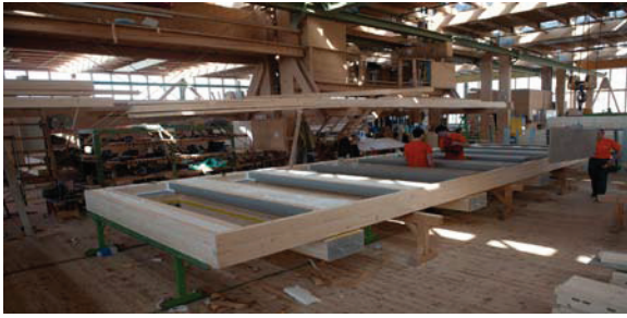
Fig 5: Production of timber frame walls
