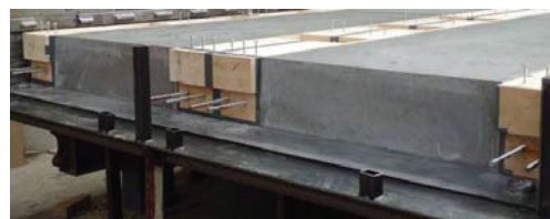
Fig.4: Production of hybrid slabs. Wood in metal frame.
