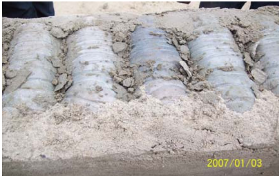
Plate 4: Waste water bottles as innovative building material
