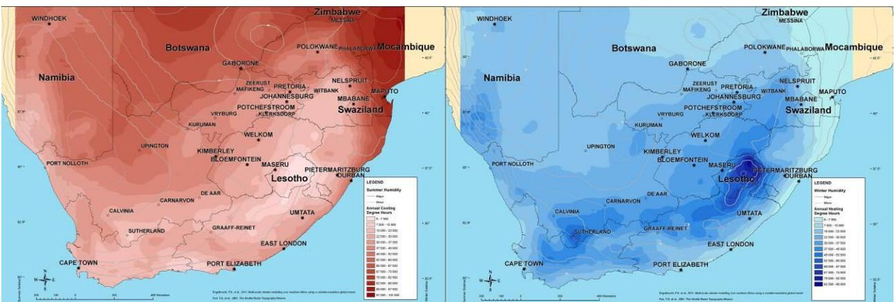
Figure 4 Separate Cooling and Heating degree maps before combination into a single map.
