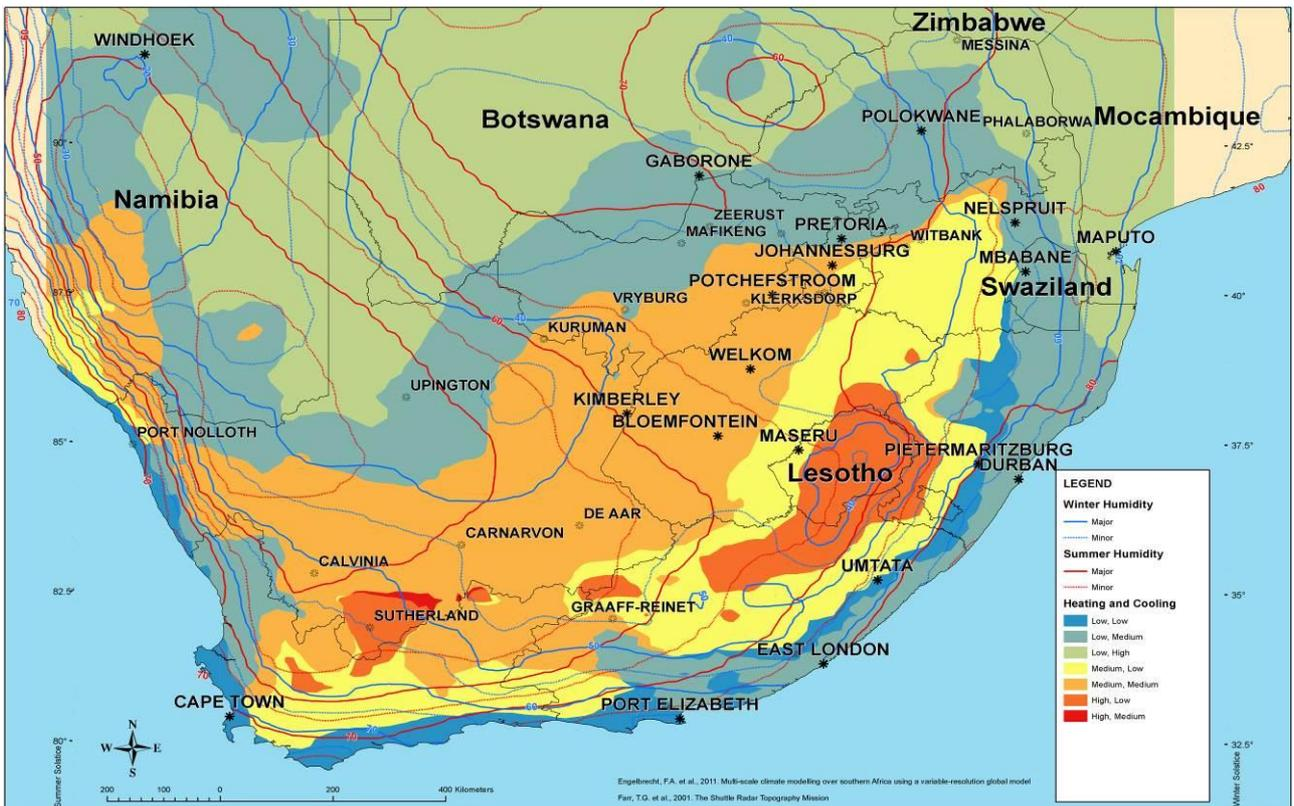
Figure 5 Heating and Cooling Degree maps combined into one map with summer and winter humidity lines.
