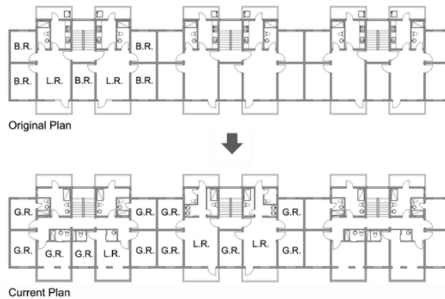
Fig. 3 Typical Plan Before and After Renovation
