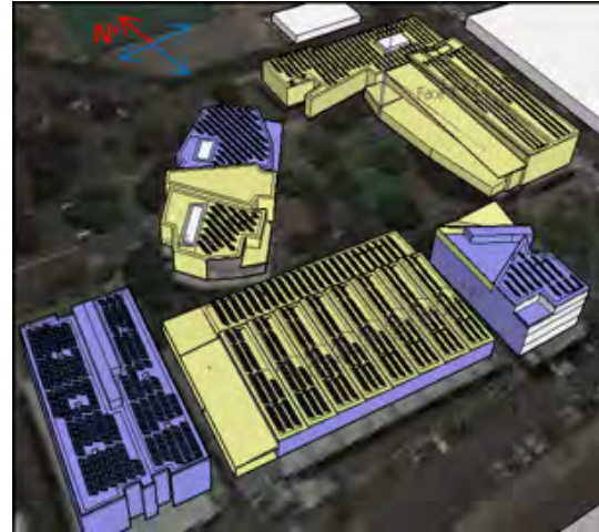
Figure 2 Solar array layout on rooftop with tilt angle of 30° and orientation of 10° East
