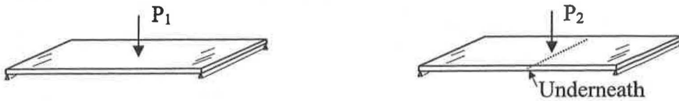
Fig.2a A simply supported glass plate Fig.2b A glass plate with a fine cut
