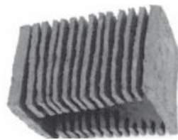
Fig. 1: Ceramic Mock-Up of »±brick« Type 2.1 dimension: 240/240/365 mm
