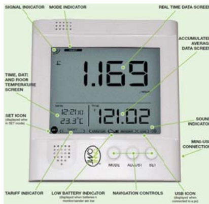
Figure 0-58: OWL metering receiver and data storage
