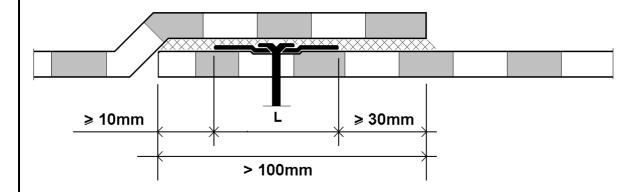
Overlap design for DUO application (self adhesive part + torched part). This is the SOPRAFIX STICK case.
