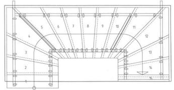
Walking line exemplified, position may be chosen freely within the walking zone, walking zone is 20 % of the clear width of the stair in the middle of the stair
